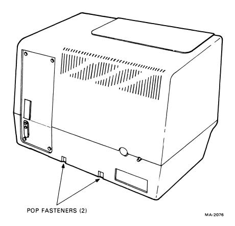
Figure 5-11b Top Cover Removal (Rear View)
