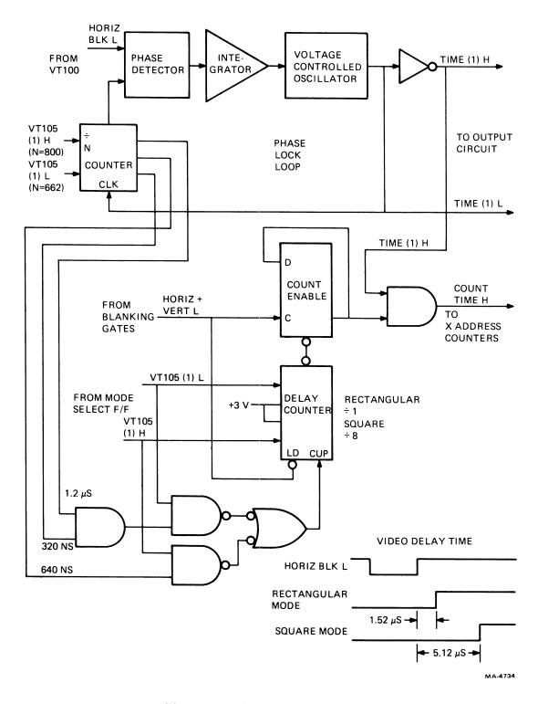
Figure 6-17 Phase Lock Loop Timing
