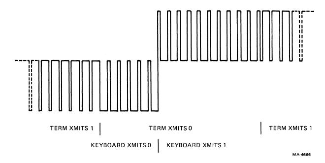
Figure 4-4-8 Keyboard Interface Signal
