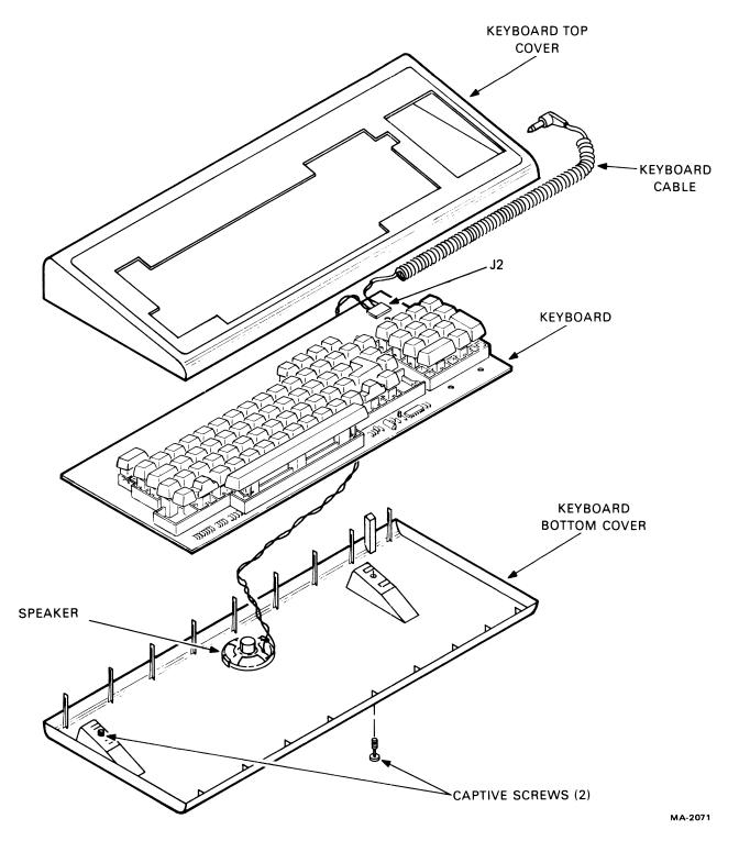
Figure 5-10 Keyboard Disassembly
