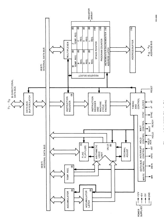
Figure 4-2-1 8080 Block Diagram
