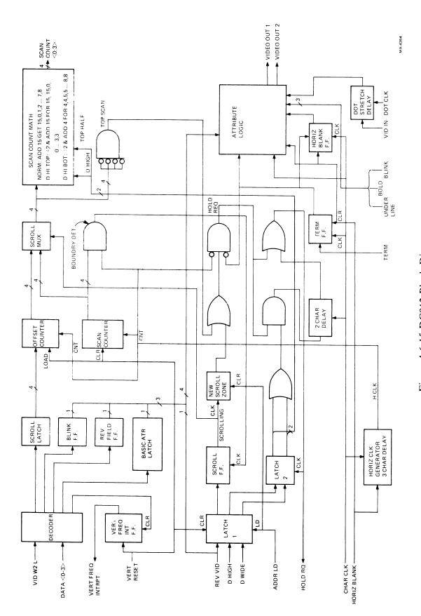
Figure 4-6-15 DC012 Block Diagram
