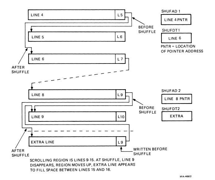
Figure 4-7-10 Split Screen Address Shuffle
