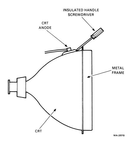
Figure 5-13 CRT Anode Discharging
