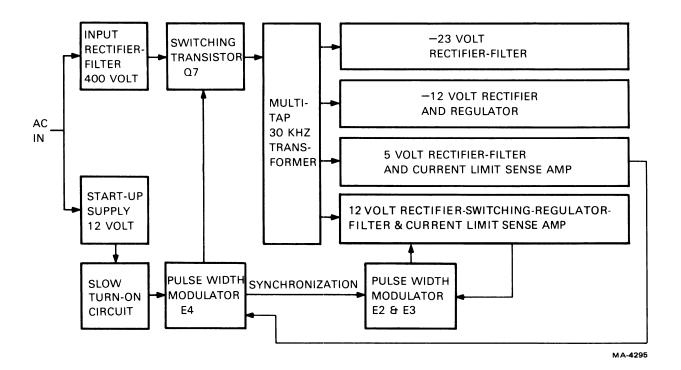
Figure 4-9-1 VT100 Power Supply Block Diagram
