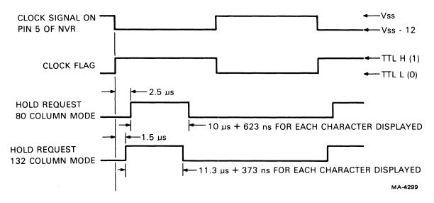
Figure 4-5-2 NVR Signals
