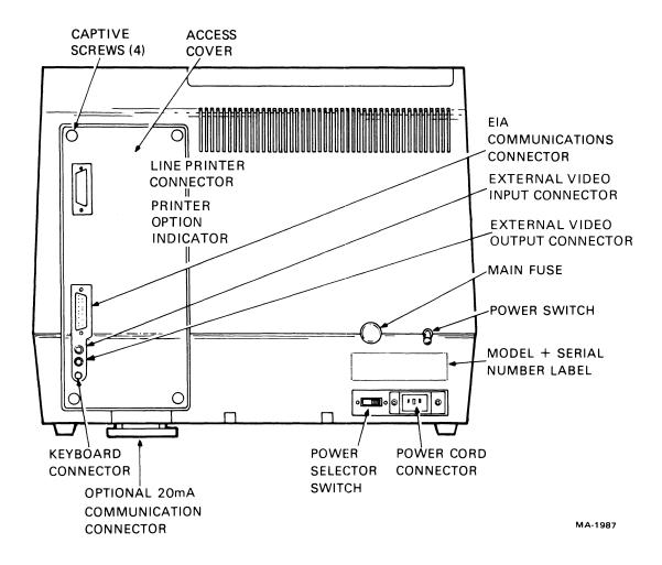
Figure 2-2 VT100 Terminal (Rear View)
