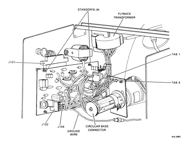
Figure 5-12 Ball Video Monitor Board Removal
