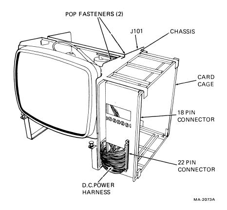
Figure 5-17 VT100 DC Power Harness Removal
