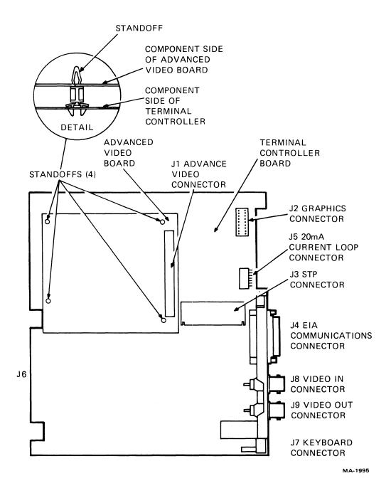
Figure 6-9 Advanced Video Option Installation
