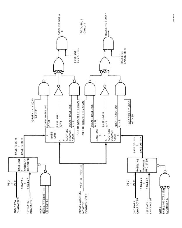
Figure 6-25 Baseline (Shade Line) Registers and Comparators
