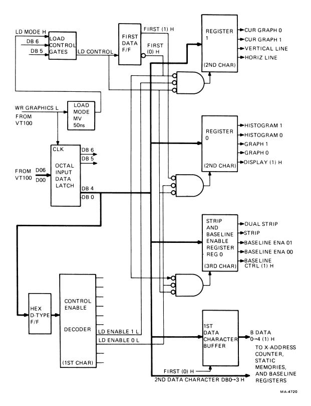
Figure 6-18 Loading the Registers
