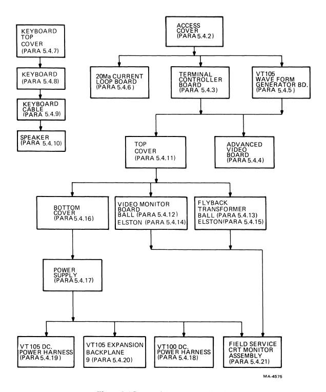
Figure 5-6 Removal Procedures Flowchart
