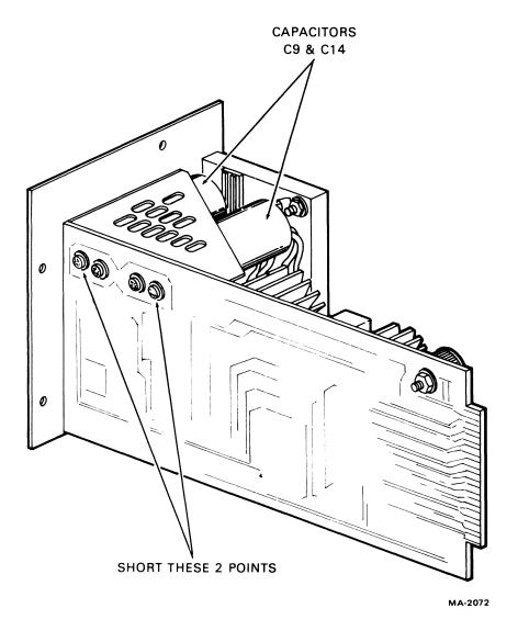
Figure 5-16 Power Supply Capacitor Discharging
