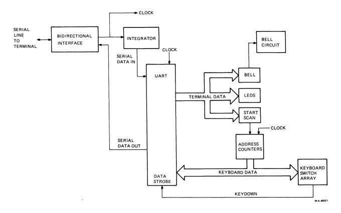
Figure 4-4-1 Keyboard Block Diagram
