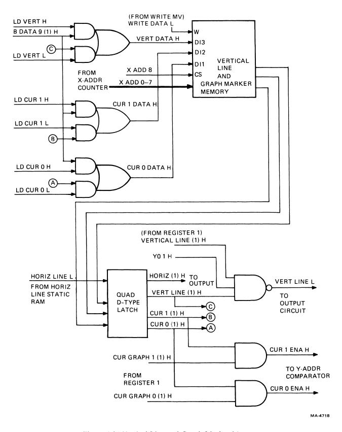
Figure 6-26 Vertical Line and Graph Marker Memory
