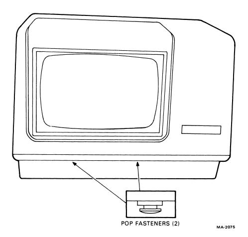
Figure 5-11a Top Cover Removal (Front View)
