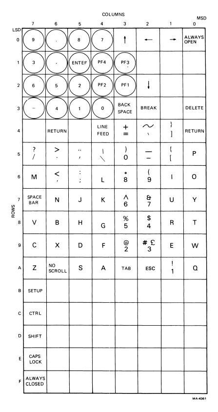
Figure 4-4-4 Keyboard Switch Array
