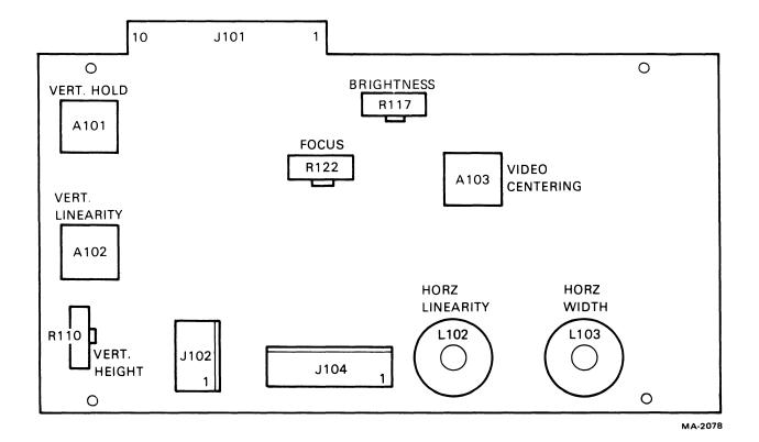
Figure 5-2 Ball Video Monitor Board Adjustments
