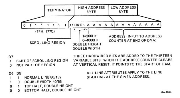
Figure 4-7-2 Terminator and Address Bytes
