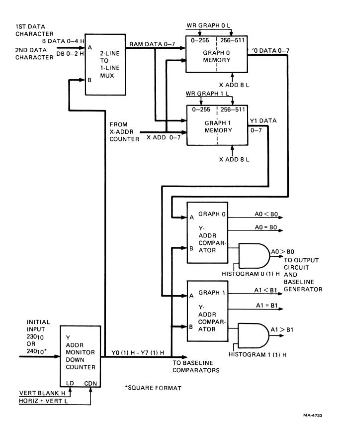
Figure 6-24 Graph Memory and Y-Address Monitor
