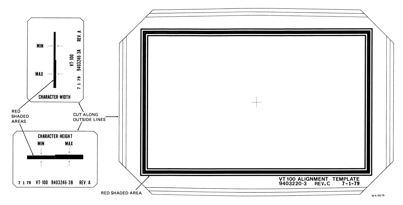
Figure 5-1 Video Alignment Templates
