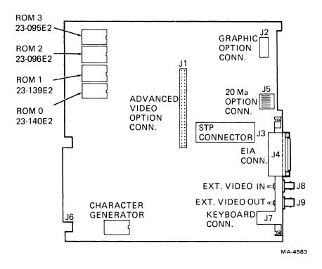
Figure 5-20 Terminal Controller Board, VT132 Configuration
