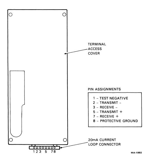
Figure 3-3 20 mA Current Loop Interface
