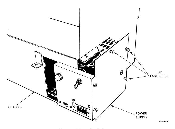
Figure 5-15 Power Supply Removal
