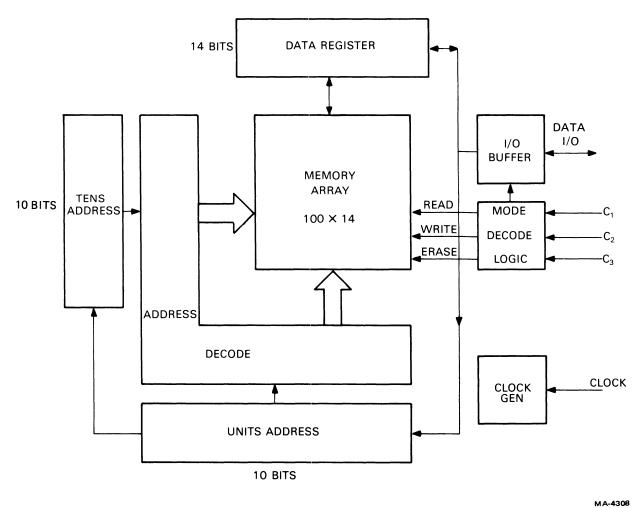
Figure 4-5-1 ER1400 NVR Block Diagram
