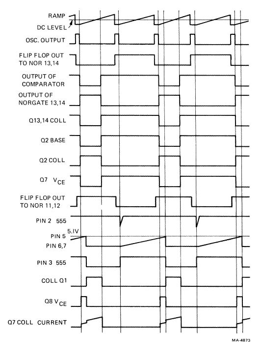
Figure 4-9-3 Power Supply Timing Diagram
