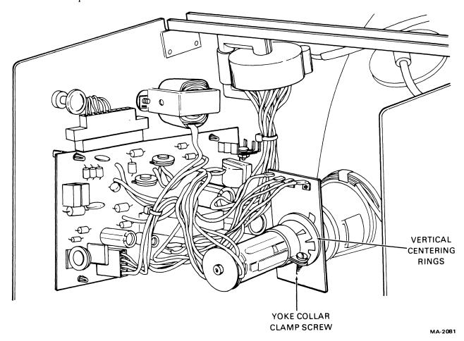
Figure 5-3 Ball Monitor CRT Adjustments
