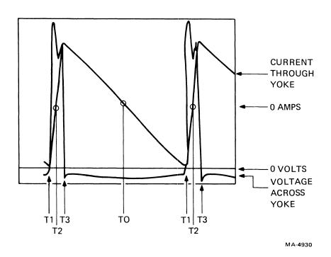
Figure 4-8-5 Horizontal Deflection Waveforms
