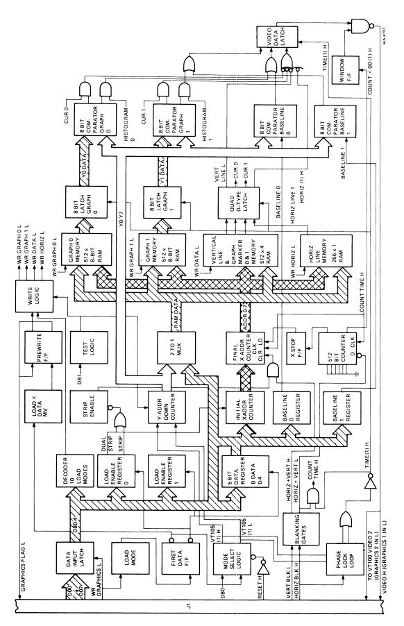
Figure 6-12 M7071 Waveform Generator Block Diagram
