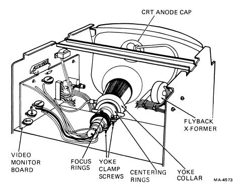
Figure 5-5 Elston Monitor CRT Adjustments
