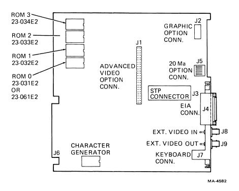
Figure 5-19 Terminal Controller Board VT100 Configuration
