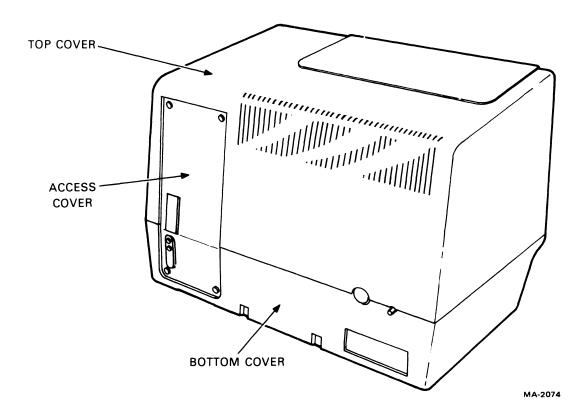
Figure 5-7 VT100 Terminal, (Rear View)
