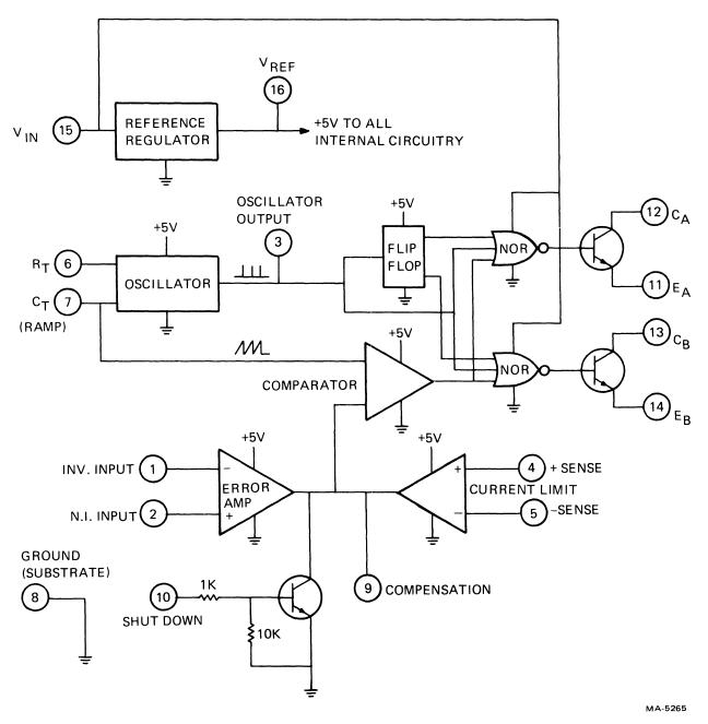
Figure 4-9-2 3524 Regulator Block Diagram
