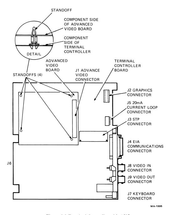
Figure 5-9 Terminal Controller with AVO
