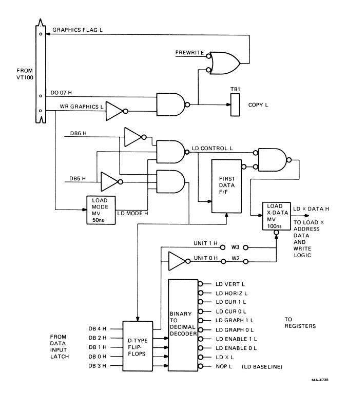
Figure 6-13 Decoding the Control Character
