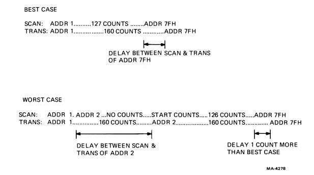
Figure 4-4-3 Key Address Transmission Delays
