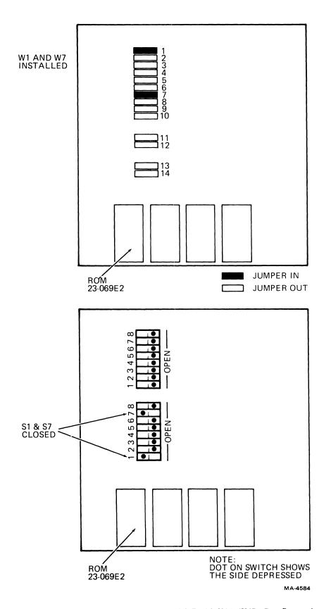
Figure 5-22 Advanced Video Board VT100-WA/WB Configuration
