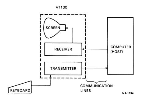
Figure A-1 Terminal Data Flow
