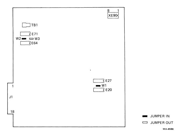
Figure 5-24 VT105 Waveform Generator Board Configuration
