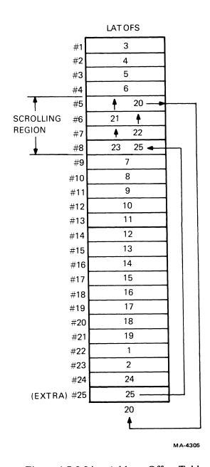
Figure 4-7-8 Line Address Offset Table
