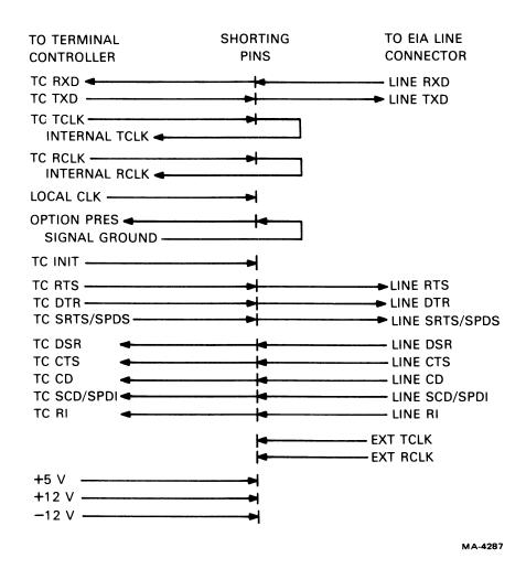
Figure 7-2 STP Signal Lines
