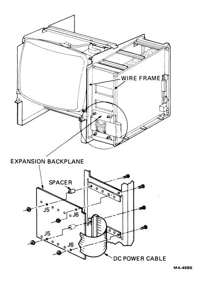
Figure 5-18 VT105 Expansion Backplane Removal
