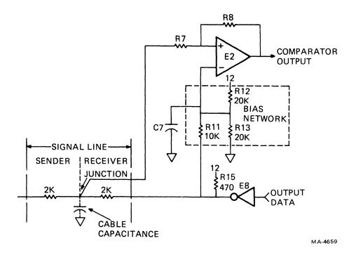
Figure 4-4-5A Keyboard Interface Circuit
