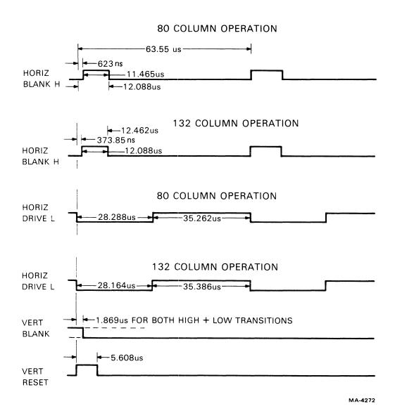
Figure 4-6-9 Horizontal Timing
