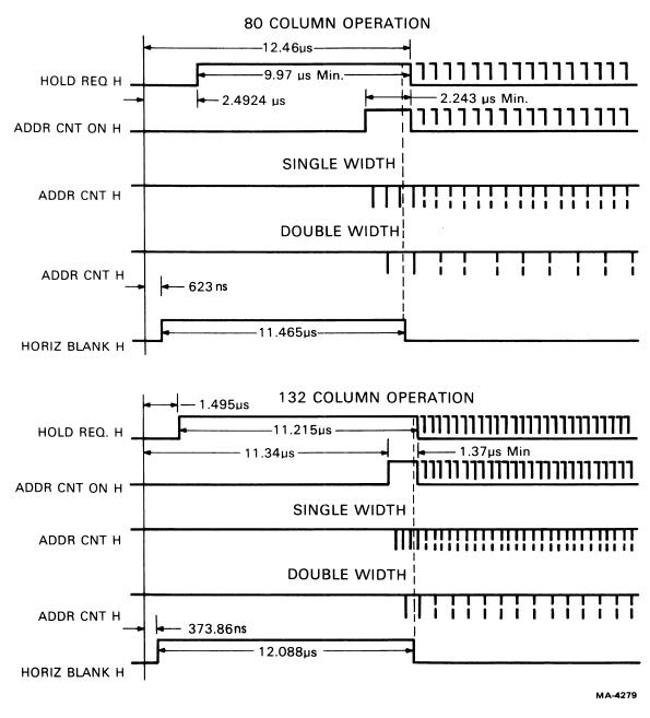
Figure 4-6-8 Address Count Timing
