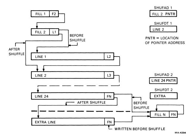
Figure 4-7-9 Full Screen Address Shuffling
