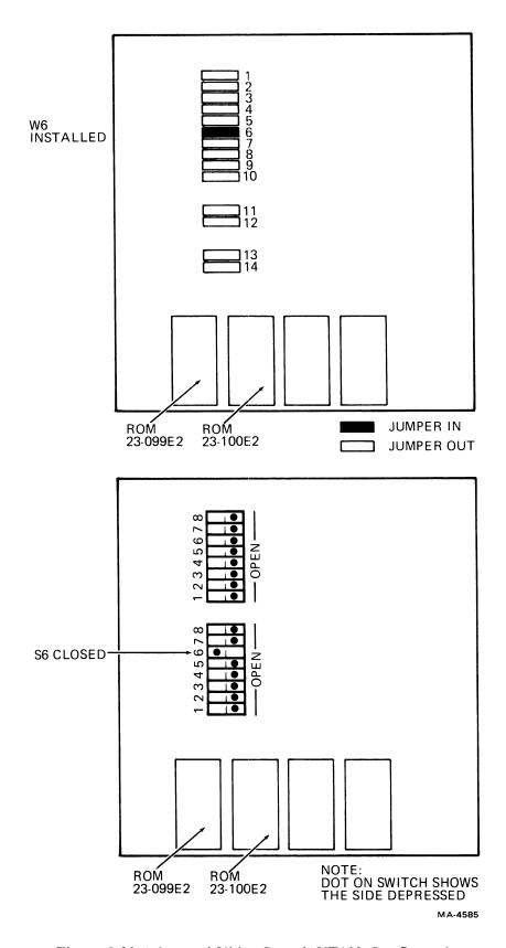
Figure 5-23 Advanced Video Board, VT132 Configuration
