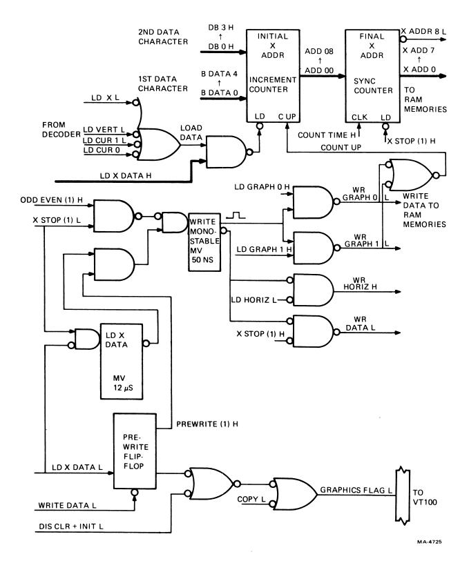
Figure 6-23 Loading Address Data
