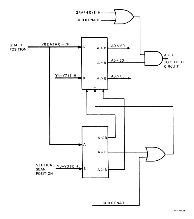
Figure 6-27 Graph Marker Y-Address Comparator
