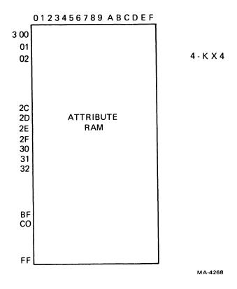
Figure 4-7-3 Screen RAM Organization – 80 Column, 60 Hz (Sheet 1 of 2)
