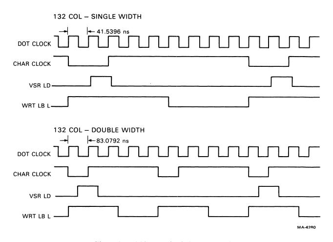
Figure 4-6-7 Video Latch Timing – 132 Column
