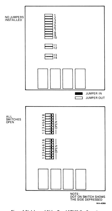
Figure 5-21 Advanced Video Board VT100 Configuration
