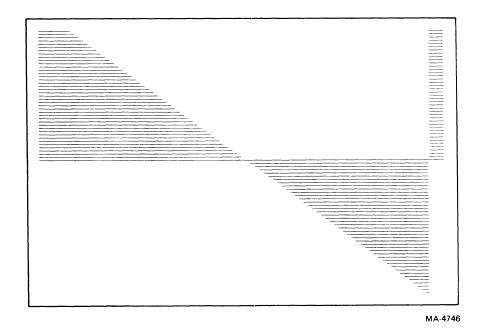
Figure 6-37 Shade Line (Baseline) Test Pattern
