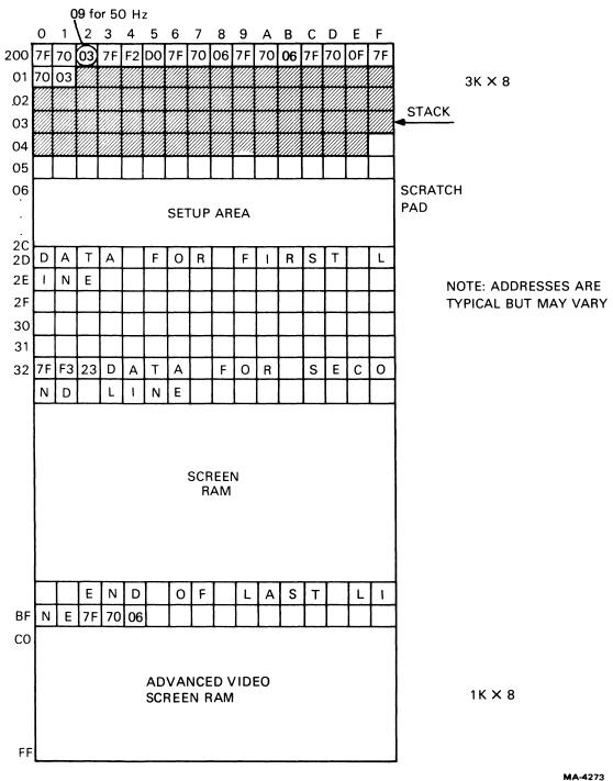
Figure 4-7-3 Screen RAM Organization - 80 Column, 60 Hz (Sheet 2 of 2)
