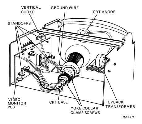
Figure 5-14 Elston Video Monitor Board Removal
