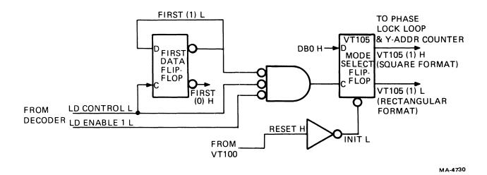
Figure 6-16 Selecting Mode of Operation
