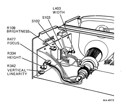
Figure 5-4 Elston Video Monitor Board Adjustments
