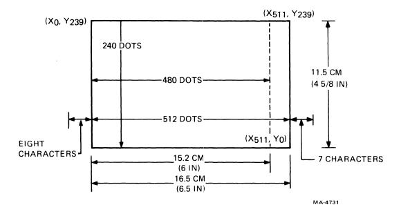
Figure 6-15 Square Aspect Ratio Graph Drawing Field
