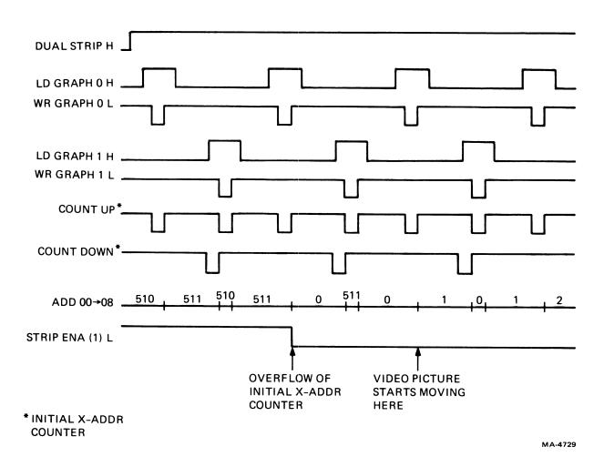
Figure 6-30 Dual Strip Chart Timing Diagram
