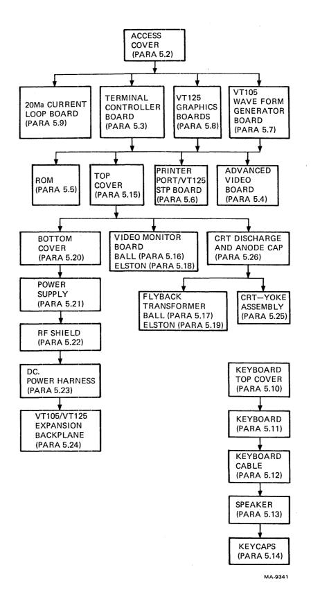
Figure 5-10 Removal Procedures Sequence
