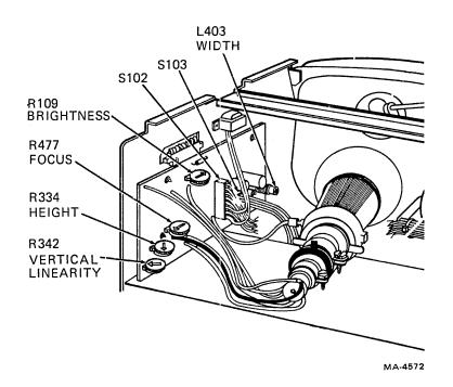
Figure 5-8 Elston Video Monitor Board Adjustments
