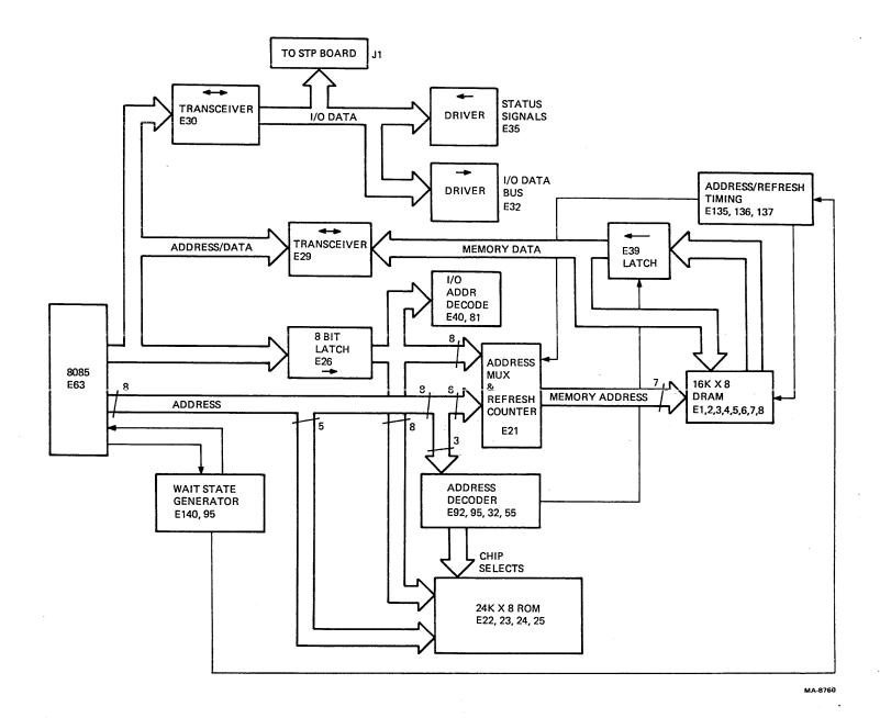
Figure 6-53 Microprocessor Address and Data Paths
