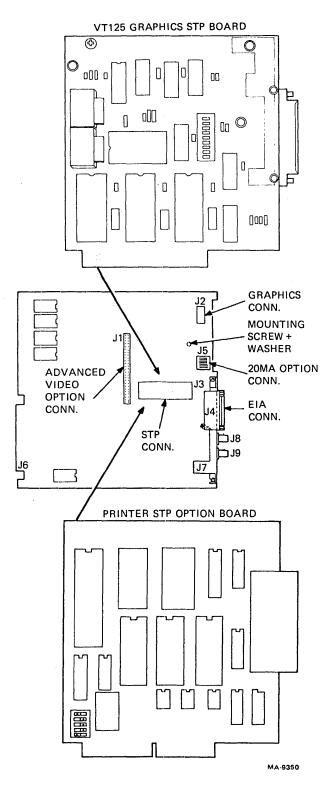
Figure 5-14 Installing Printer Port on VT125 STP Board
