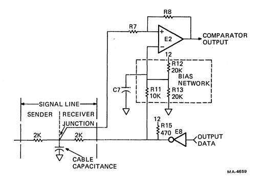
Figure 4-4-5A Keyboard Interface Circuit
