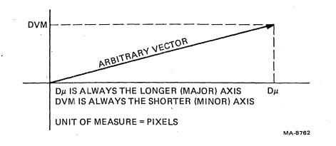
Figure 6-62 Derivation of  $D\mu$  and DVM
