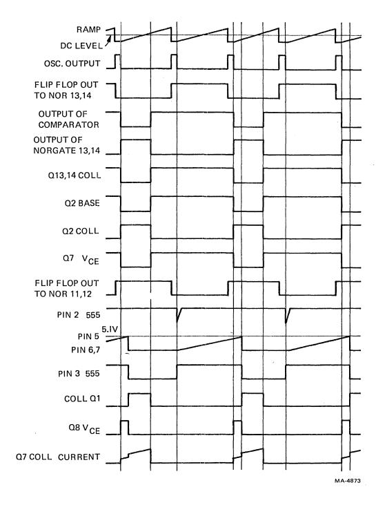
Figure 4-9-3 Power Supply Timing Diagram
