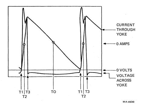
Figure 4-8-5 Horizontal Deflection Waveforms
