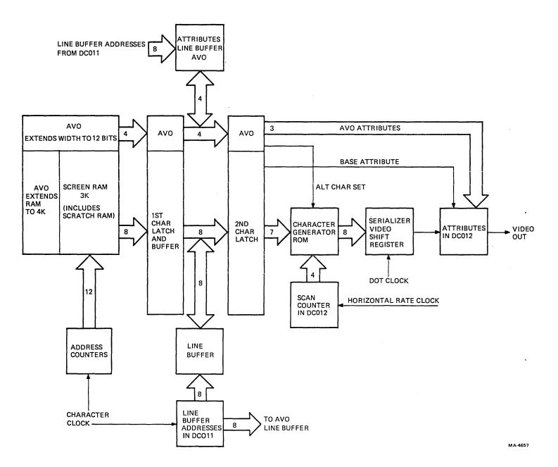
Figure 4-6-3 Video Processor Functional Diagram
