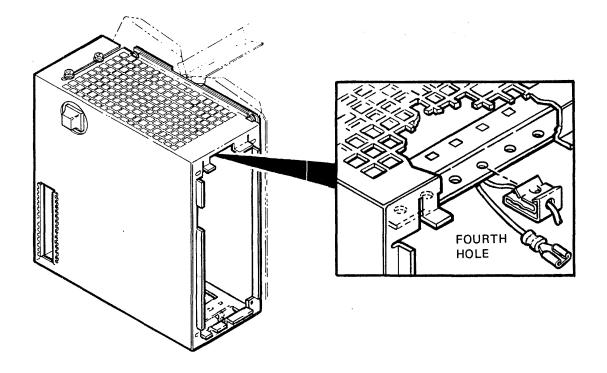
NOTE: INSTALL CLIP BEFORE INSTALLING SHIELD.
