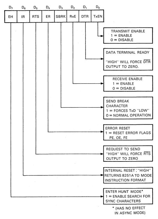
NOTE: ERROR RESET MUST BE PERFORMED WHENEVER RXENABLE AND ENTER HUNT ARE PROGRAMMED.
