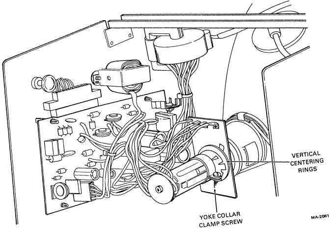
Figure 5-7 Ball Monitor CRT Adjustments
