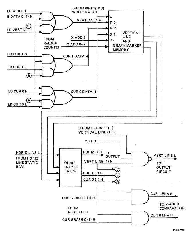
Figure 6-30 Vertical Line and Graph Marker Memory
