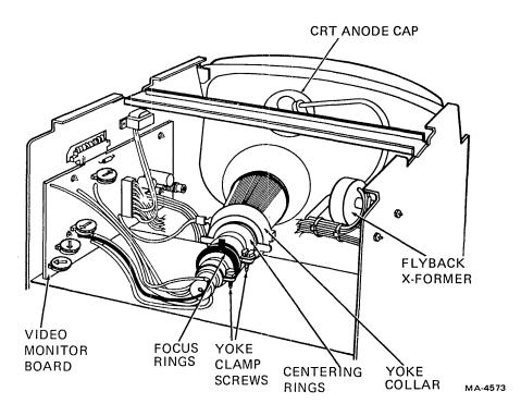
Figure 5-9 Elston Monitor CRT Adjustments
