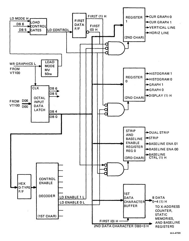
Figure 6-22 Loading the Registers
