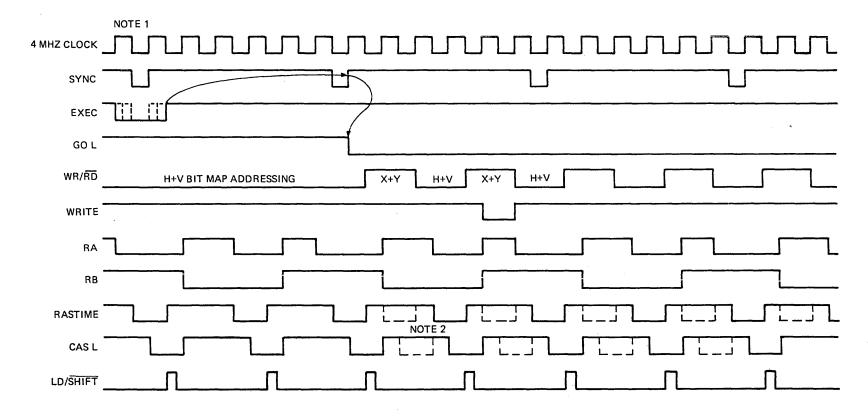
NOTE 1 SIGNALS ARE LATCHED BY 8 MHZ. 1/2 CYCLE SHIFT NOT SHOWN. NOTE 2 DOTTED SIGNALS SHOW ADDED BIT MAP MEMORY ACCESSES WHEN VECTOR GENERATOR IS RUNNING.
