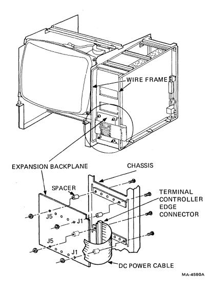
Figure 6-44 Installing Expansion Backplane
