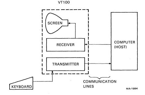
Figure A-1 Terminal Data Flow
