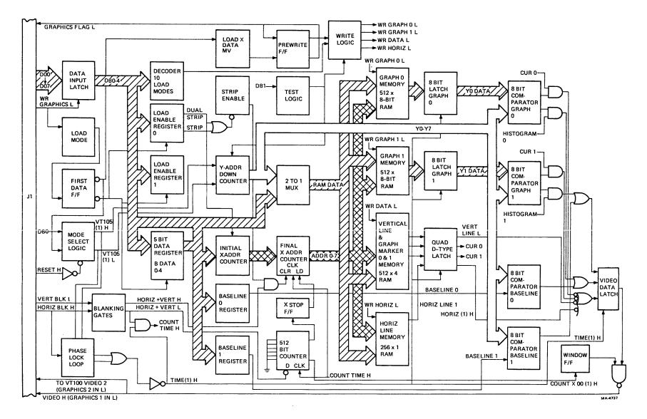
Figure 6-16 M7071 Waveform Generator Block Diagram
