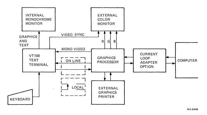
Figure 5-1 VT125 General Block Diagram
