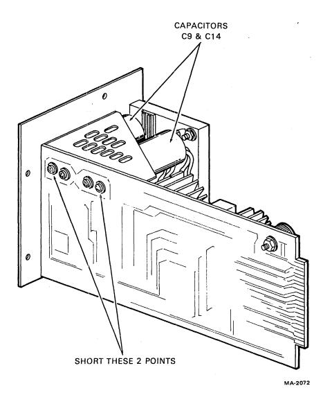
Figure 5-25 Power Supply Capacitator Discharging
