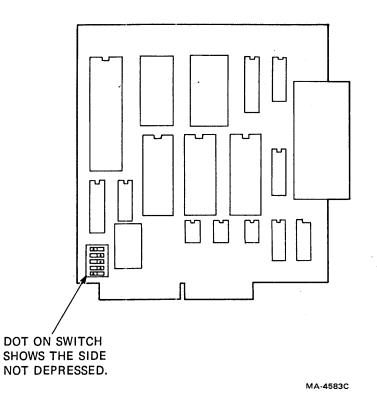
Figure 5-35 VT1XX-AC Printer Port Option Board
