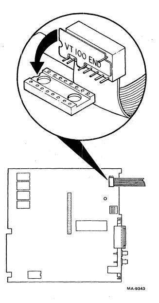
Figure 6-46 16-Pin Flat Cable on Terminal Controller
