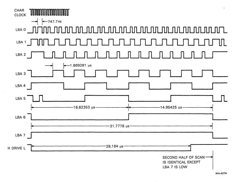
Figure 4-6-11 Line Buffer Address Outputs - 132 Column
