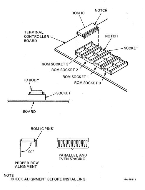
Figure 5-13 Terminal Controller Board ROM Installation
