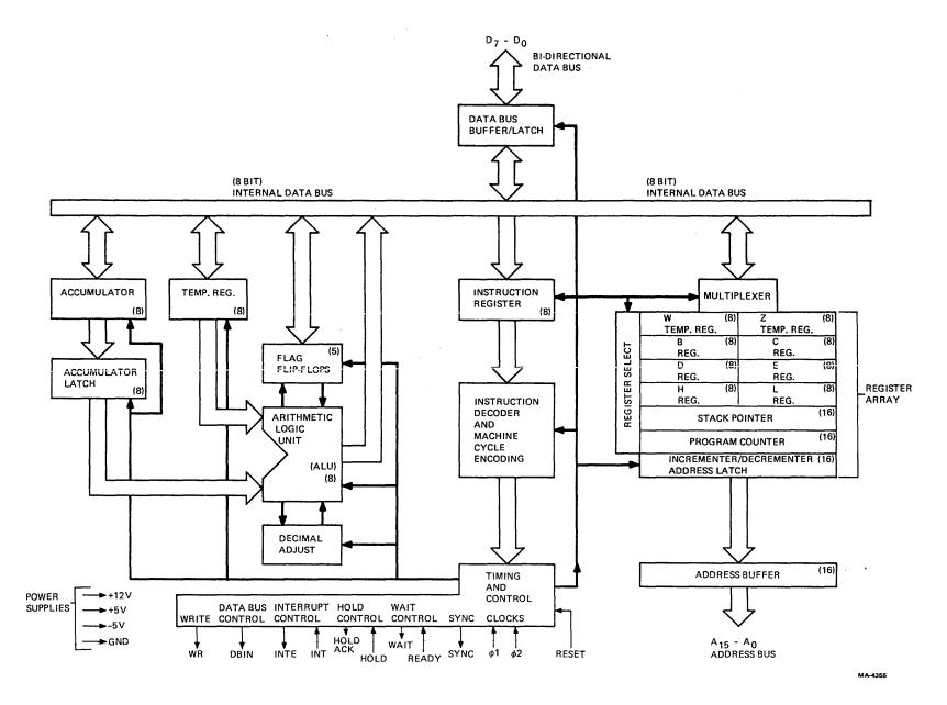
Figure 4-2-1 8080 Block Diagram
