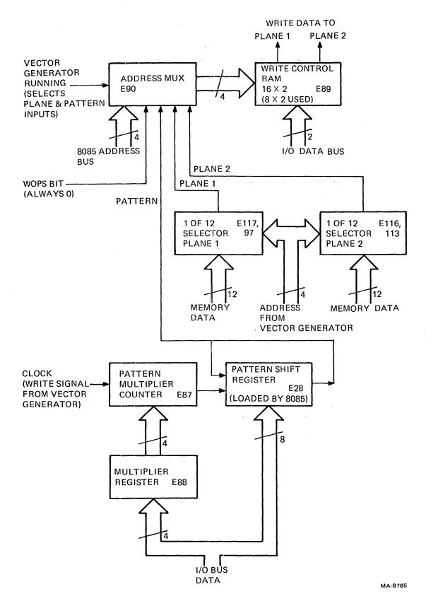
Figure 6-71 Bit Map Write Control Block Diagram
