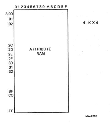
Figure 4-7-3 Screen RAM Organization – 80 Column, 60 Hz (Sheet 1 of 2)
