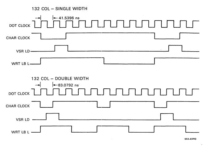
Figure 4-6-7 Video Latch Timing - 132 Column
