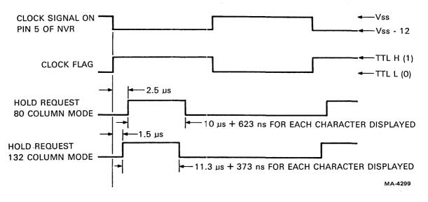
Figure 4-5-2 NVR Signals
