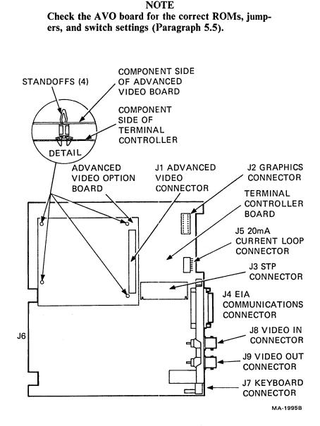
Figure 5-12 Terminal Controller with Advanced Video Board
