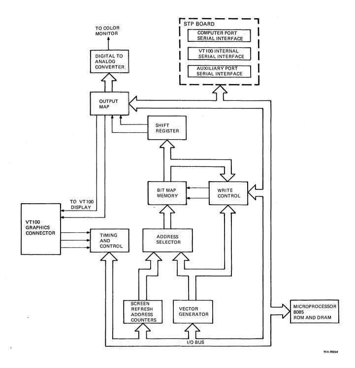
Figure 6-52 VT125 Graphics Processor Block Diagram
