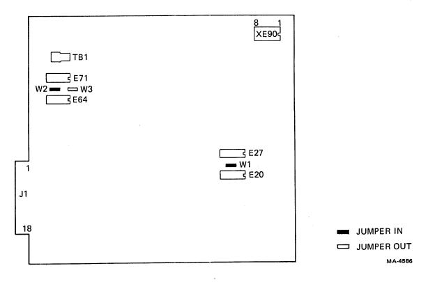
Figure 5-36 VT105 Waveform Generator Board
