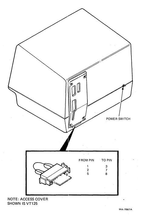
Figure 5-3 20 mA Loopback Connector
