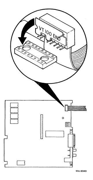
Figure 5-17 VT125 16-Pin Flat Cable on Terminal Controller
