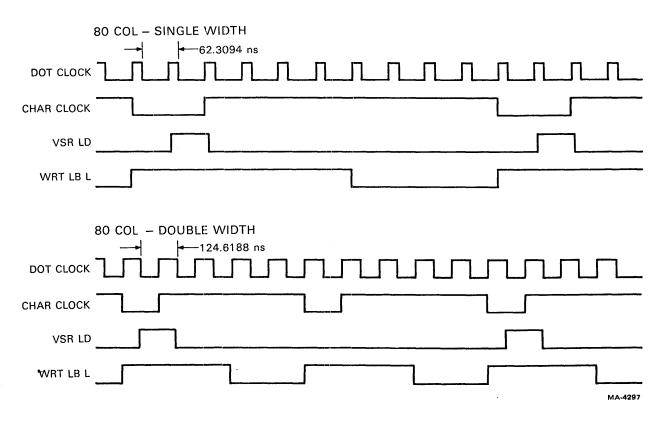
Figure 4-6-6 Video Latch Timing – 80 Column
