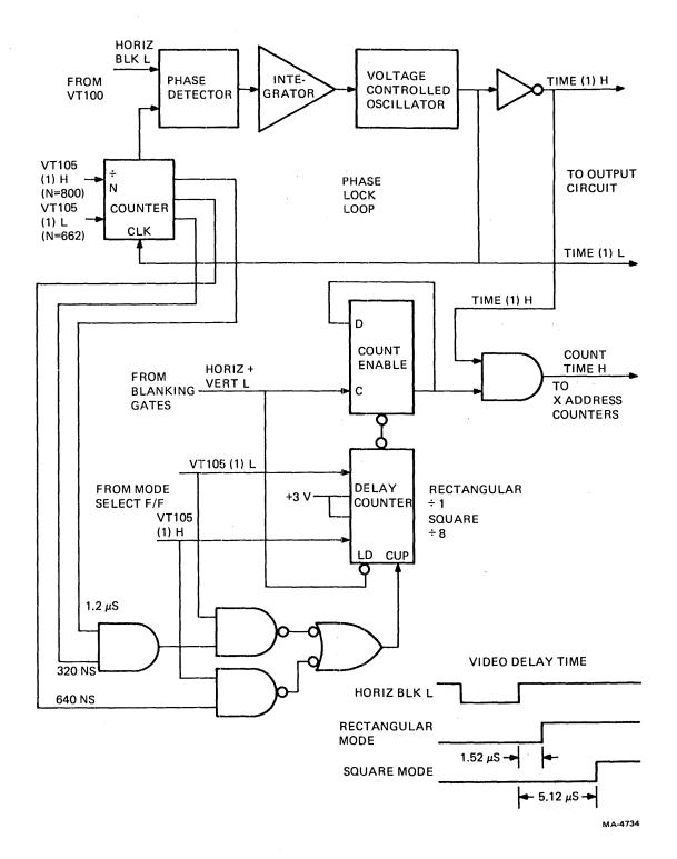
Figure 6-21 Phase-Lock-Loop Timing
