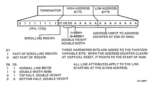
Figure 4-7-2 Terminator and Address Bytes
