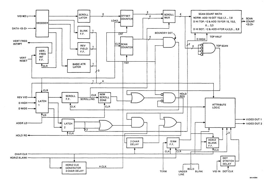
Figure 4-6-15 DC012 Block Diagram
