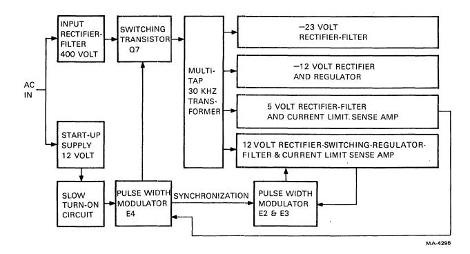
Figure 4-9-1 VT100 Power Supply Block Diagram
