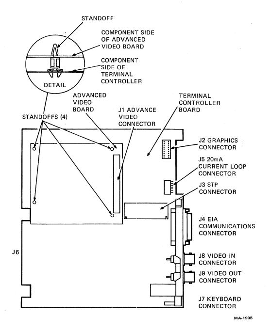
Figure 6-13 Advanced Video Option Installation
