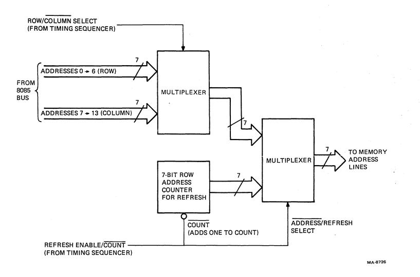
Figure 6-56 Address Multiplexer and Refresh Counter
