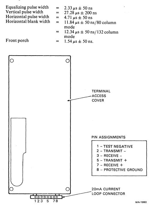
Figure 3-3 20 mA Current Loop Interface
