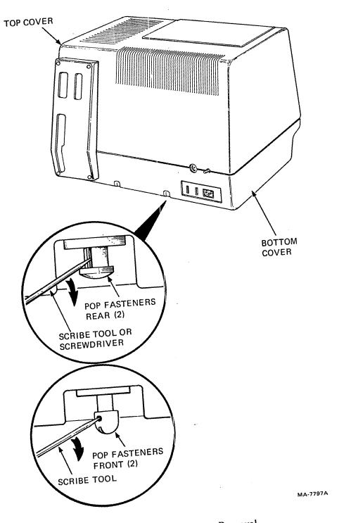
Figure 5-21 Top Cover Removal
