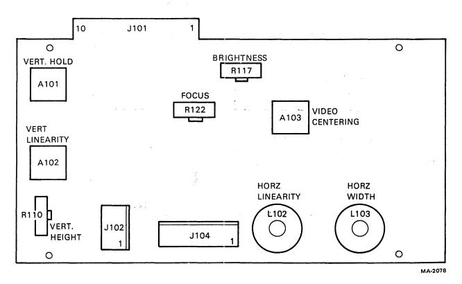
Figure 5-6 Ball Video Monitor Board Adjustments
