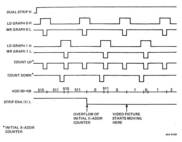
Figure 6-34 Dual Strip Chart Timing Diagram
