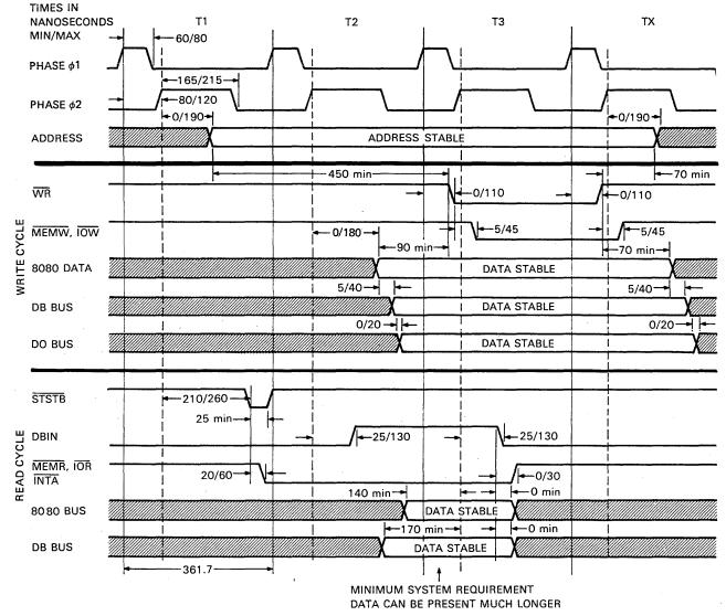
Figure 4-2-3 Microprocessor Bus Timing
