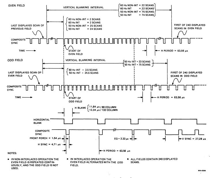
Figure 4-6-14 Composite Sync Output
