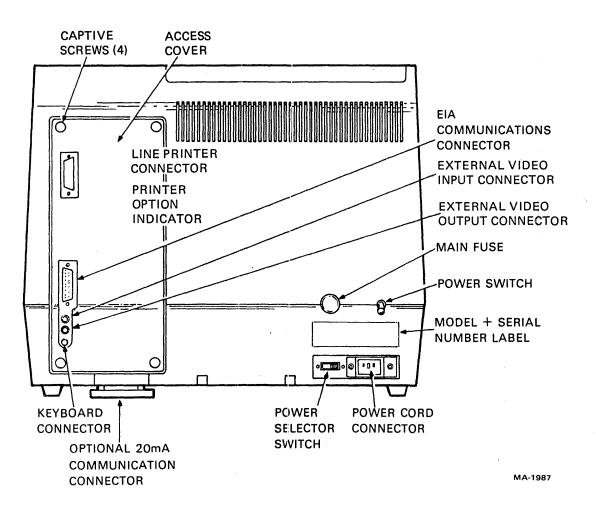
Figure 2-2 VT100 Terminal (Rear View)
