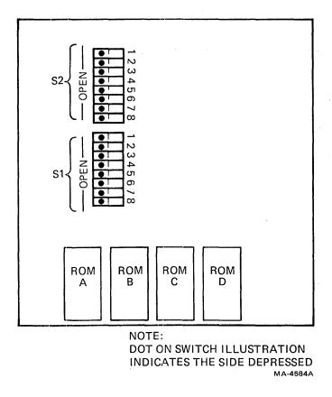
Figure 5-34 Advanced Video Option Board with Switches
