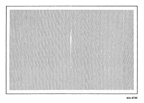
Figure 6-39 Horizontal Lines Test Pattern
