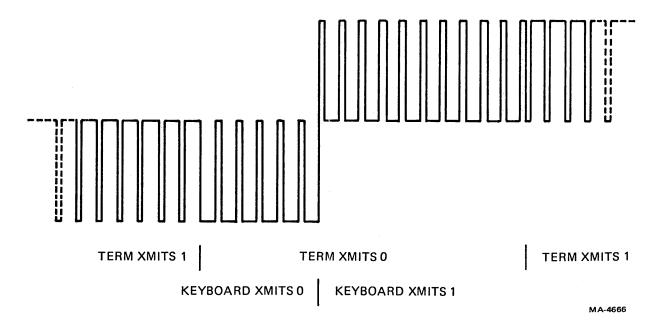
Figure 4-4-8 Keyboard Interface Signal
