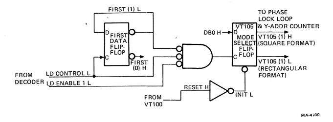
Figure 6-20 Selecting Mode of Operation
