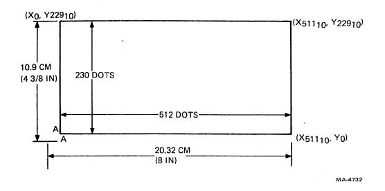
Figure 6-18 Rectangular Aspect Ratio Graph Drawing Field
