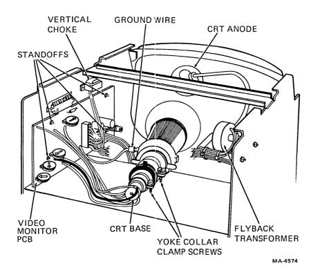
Figure 5-23 Elston/DIGITAL Video Monitor Board Removal
