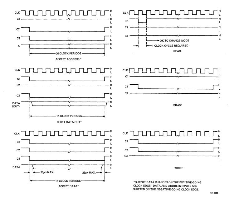
Figure 4-5-3 NVR Timing Diagrams
