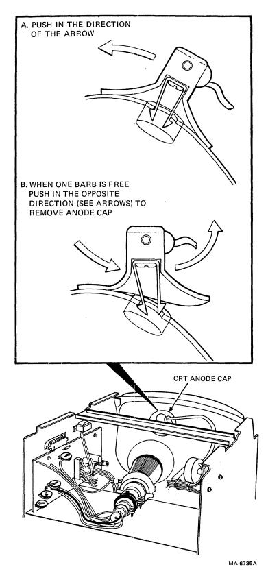
Figure 5-30 Removing Anode Cap
