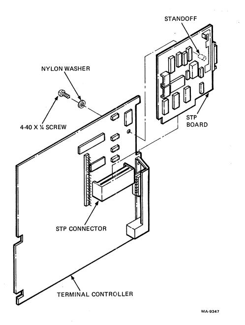
Figure 6-47 Installing STP Board
