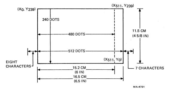
Figure 6-19 Square Aspect Ratio Graph Drawing Field
