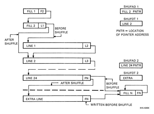
Figure 4-7-9 Full Screen Address Shuffle
