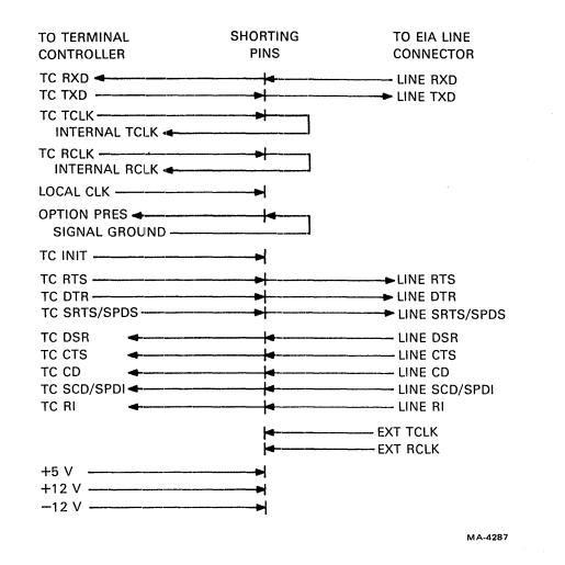
Figure 7-2 STP Signal Lines
