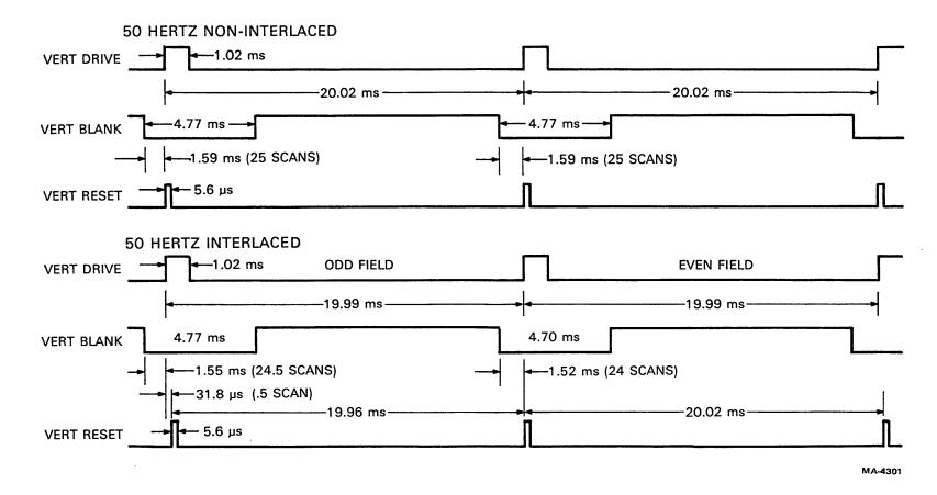
Figure 4-6-13 Vertical Signals - 50 Hz
