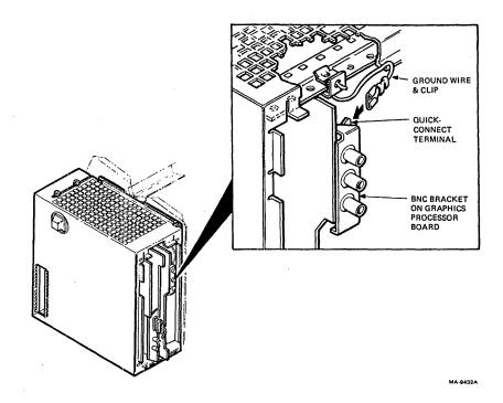
Figure 6-51 Connecting BNC Bracket Ground Wire
