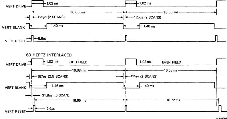
Figure 4-6-12 Vertical Signals - 60 Hz
