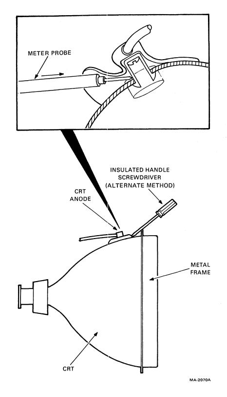
Figure 5-29 CRT Anode Discharging
