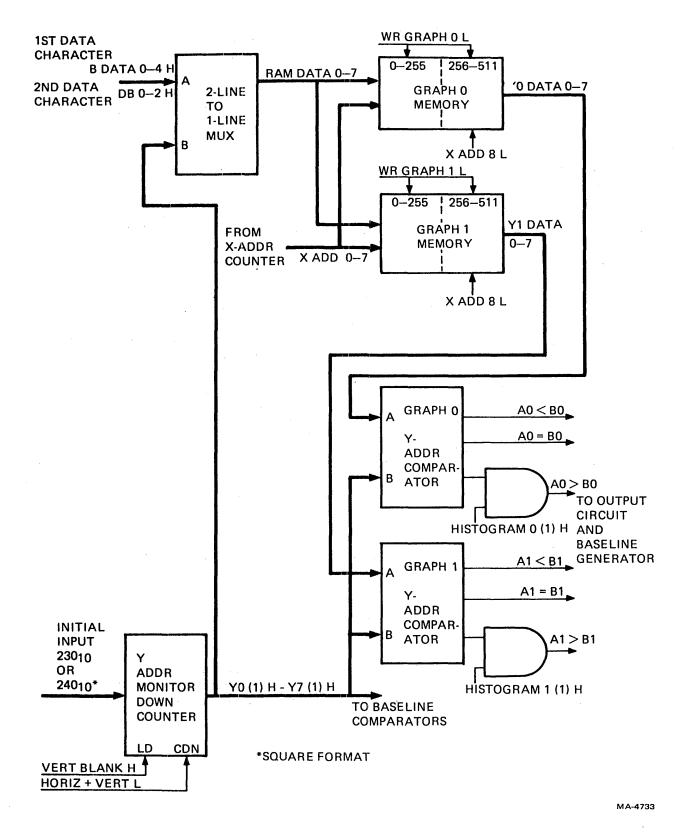
Figure 6-28 Graph Memory and Y-Address Monitor
