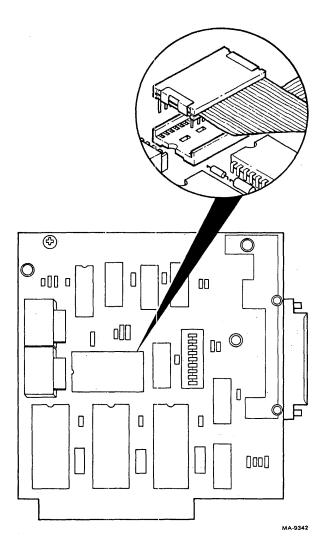
Figure 5-15 VT125 24-Pin Flat Cable on STP Board
