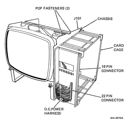
Figure 5-27 VT100 DC Power Harness Removal
