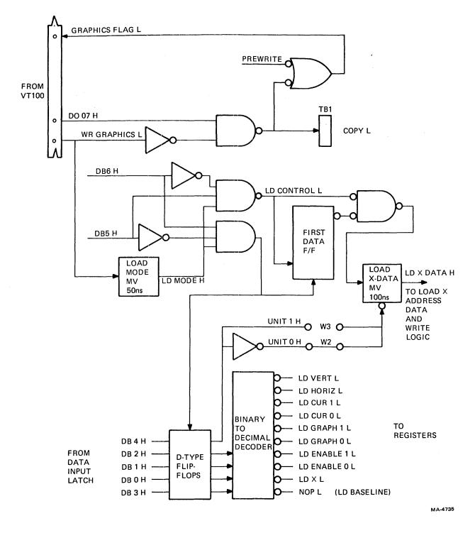
Figure 6-17 Decoding the Control Character
