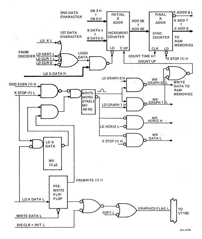
Figure 6-27 Loading Address Data
