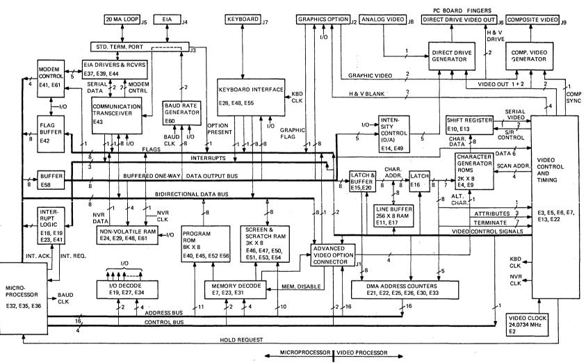
Figure 4-2-2 Microprocessor Block Diagram
