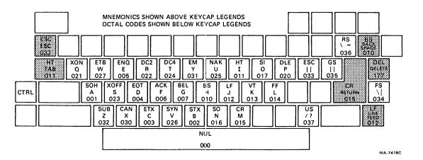
Figure A-4 Function Key Control Codes
