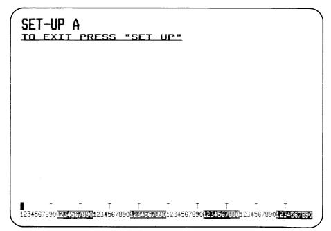
Figure 1-4 SET-UP A Mode Presentation **SET-UP B** – SET-UP B mode may only be entered from SET-UP A mode. To enter SET-UP B from SET-UP A, press the **5** key on the main keyboard. The display will then look like Figure 1-5.
