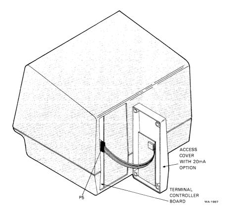
Figure 4-4 Terminal Controller Board
