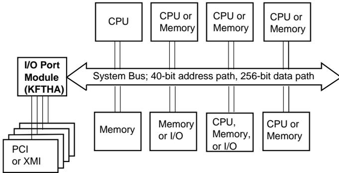
The AlphaServer 8400 has a nine-slot system bus. The minimum system configuration is one CPU module (with one or two CPUs), one memory module, and one I/O adapter. The I/O adapter shown here is the KFTHA. The remaining slots in the backplane can be used for CPU, memory, or KFTHA or KFTIA I/O adapters, within the following limits:
