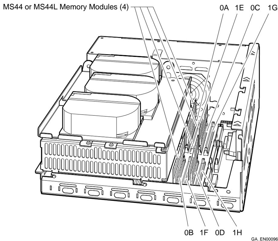
3. Push the metal board clips on the memory module connector away from the center. Tilt the memory module towards the back of the enclosure, and lift the memory module out of its connector (see Figure 3–5).
