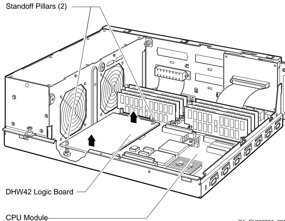
2. Press the latch on the other standoff pillar and push up the corner of the DHW42 logic board until the latch releases the DHW42 logic board.
