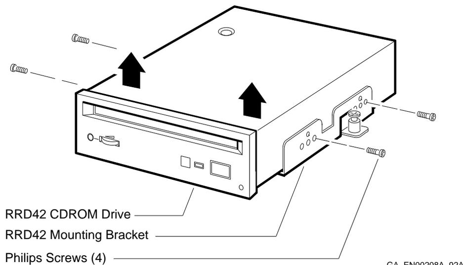
3. Keep the mounting bracket and the four screws in a safe place because you must use the same bracket and screws to install the replacement RRD42 CD-ROM drive.
