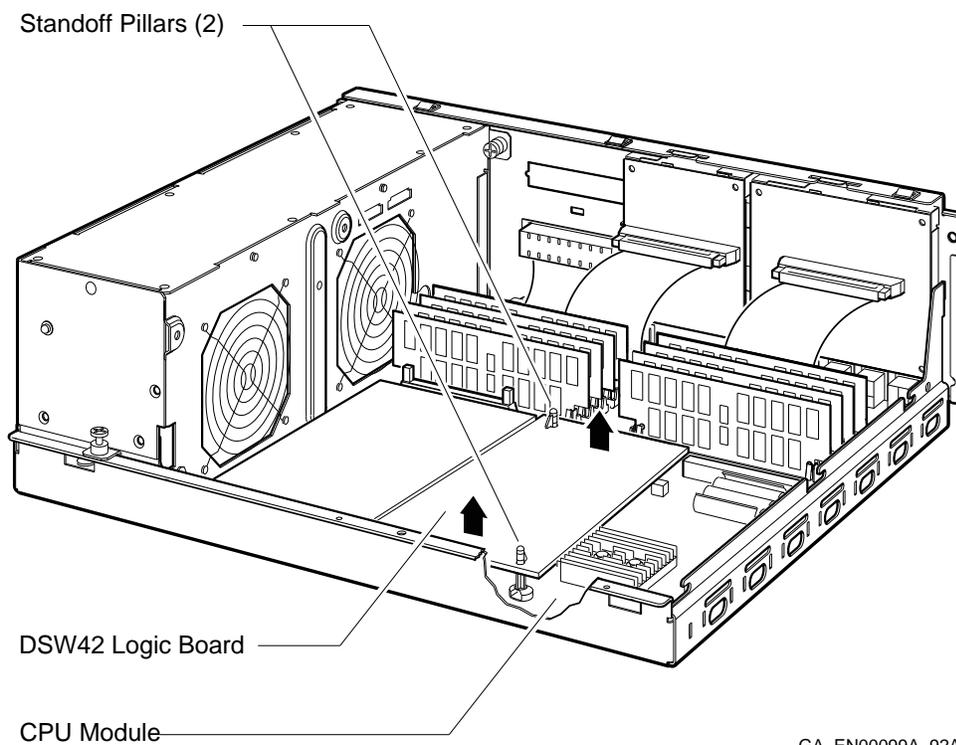
2. Press the latch on the other standoff pillar and push up that corner of the DSW42 logic board until the DSW42 logic board is released.
