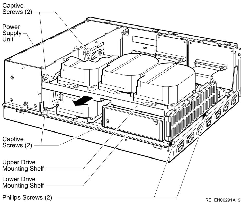
5. Slide the upper and lower drive-mounting shelf combination towards the front of the enclosure as far as it will go.
