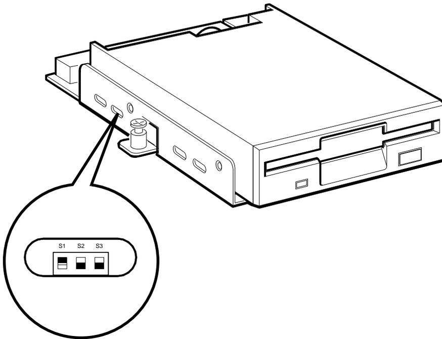
Note: The SCSI ID shown is 4 (S1 is on, S2 is off, and S3 is off).
