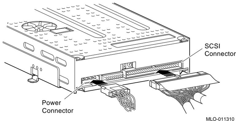
4. Loosen the captive screw on the mounting bracket that secures the drive in place and remove the drive. Figure 3–20 shows the installation of a drive in the right storage slot of the lower drive-mounting shelf.
