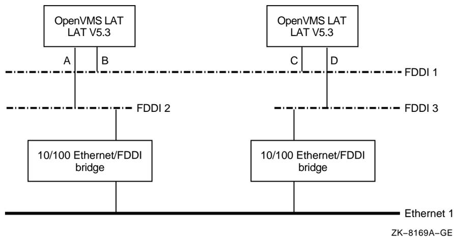
In this diagram, it is possible for the two OpenVMS systems to communicate using large packets through the path described by controllers B and C. *Large* packets may exceed 1500 bytes of data (the maximum Ethernet message can contain 1500 bytes of data). If the path described by controllers B and C were to fail, it will not be possible for communication to continue through the path described by A and D.
