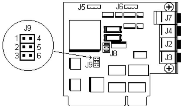
**Figure 2-5. AlphaStation 200 Series System Sound Card Jumpers**
