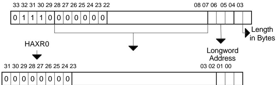
**Figure 3-4. PCI Sparse I/O Space Translation (Lower 256 KBytes)**
