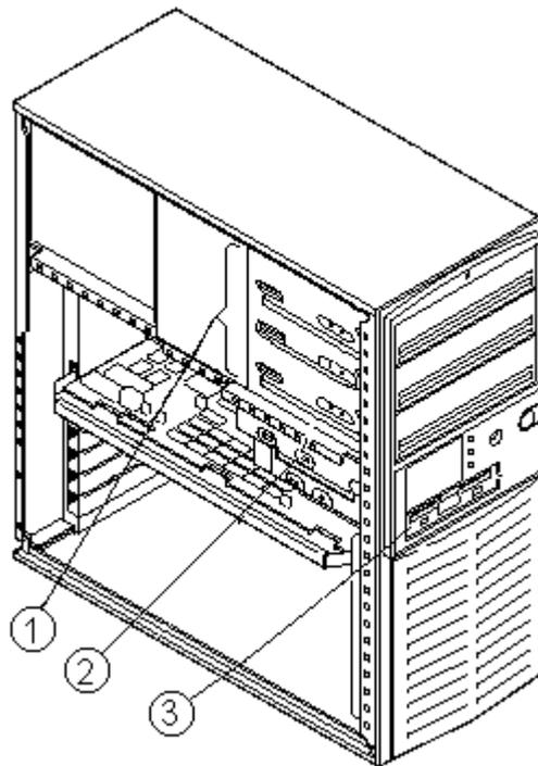
**Figure 2-2. Internal Bays - AlphaStation 400 Series Systems**
