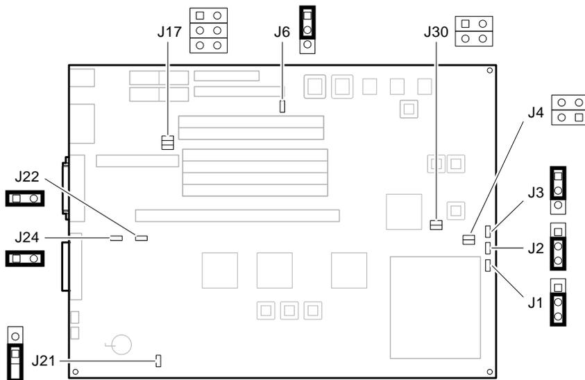
Figure 2-4. AlphaStation 200 Series System Motherboard Jumpers
