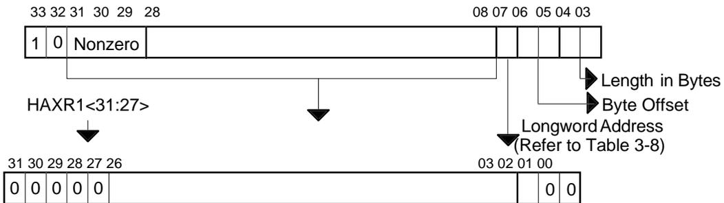
**Figure 3-9. PCI Memory Space Address Translation (Remaining 112 MBytes)**
