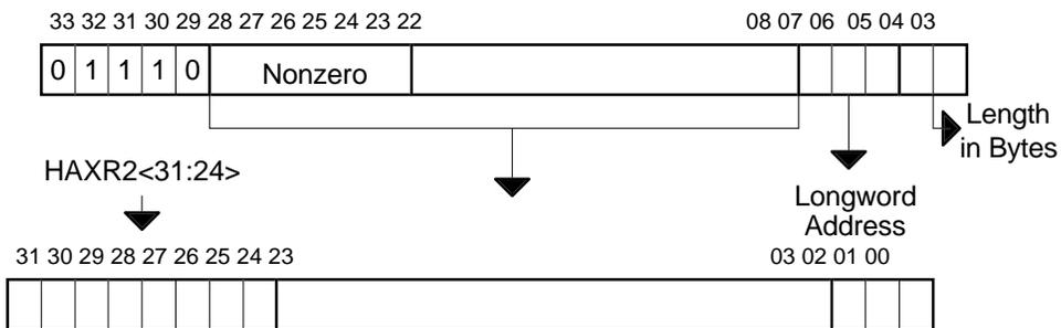
**Figure 3-5. PCI Sparse I/O Address Translation (Remaining 16 MBytes)**
