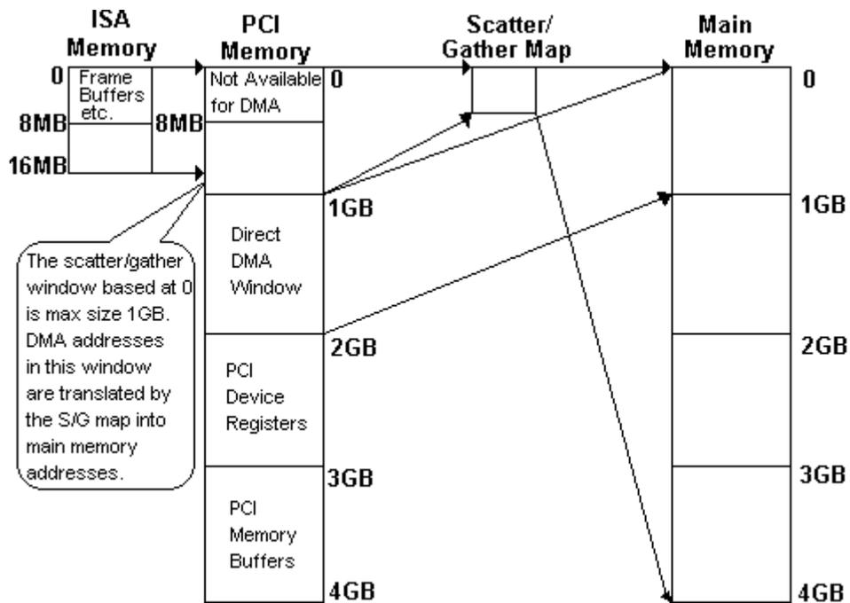
Figure 3-11. Address Space from the I/O Perspective
