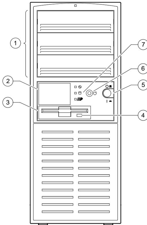
**Figure 1-3. AlphaStation 400 Series Control and Indicators**
