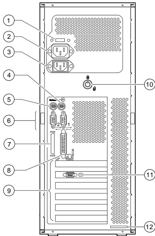
**Figure 10-2. AlphaStation 400 Series System Rear Connectors**
