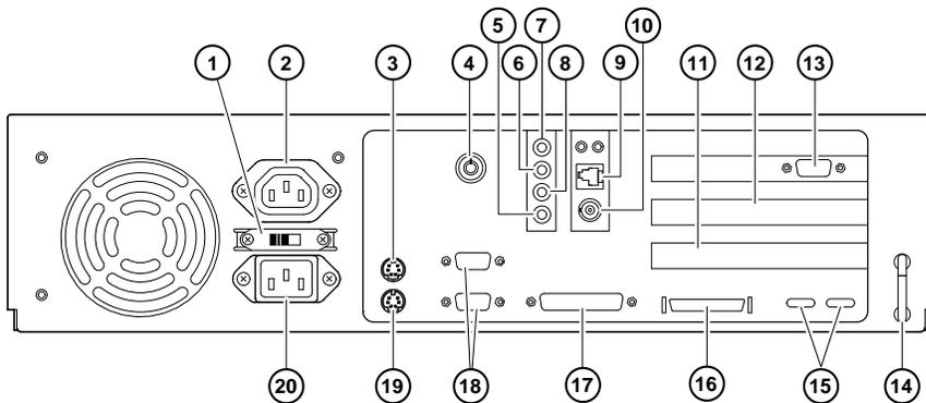
**Figure 10-1. AlphaStation 200 Series System Rear Connectors**
