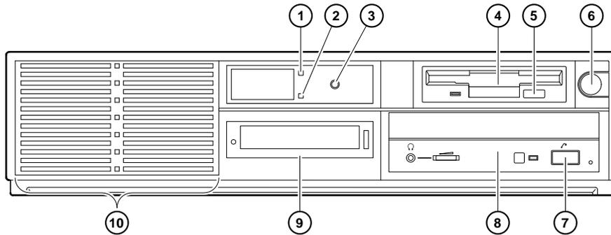
**Figure 1-1. AlphaStation 200 Series Control and Indicators**
