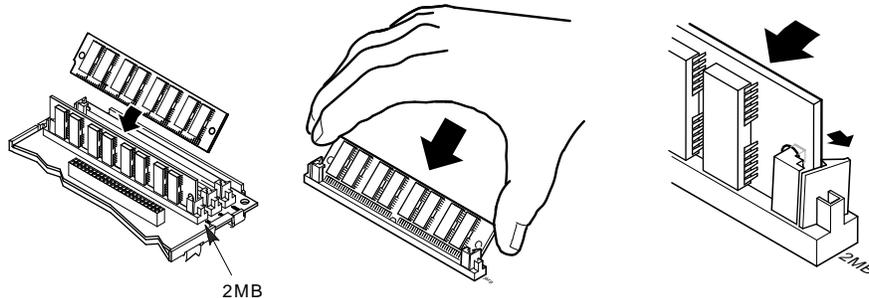
**To remove the SIMM card:** Gently push outward on the tabs at the sides of the connector. Tilt the SIMM card toward the edge of the image board at a 45-degree angle. Grasp the edges of the SIMM card firmly and lift the card out of the connector.
