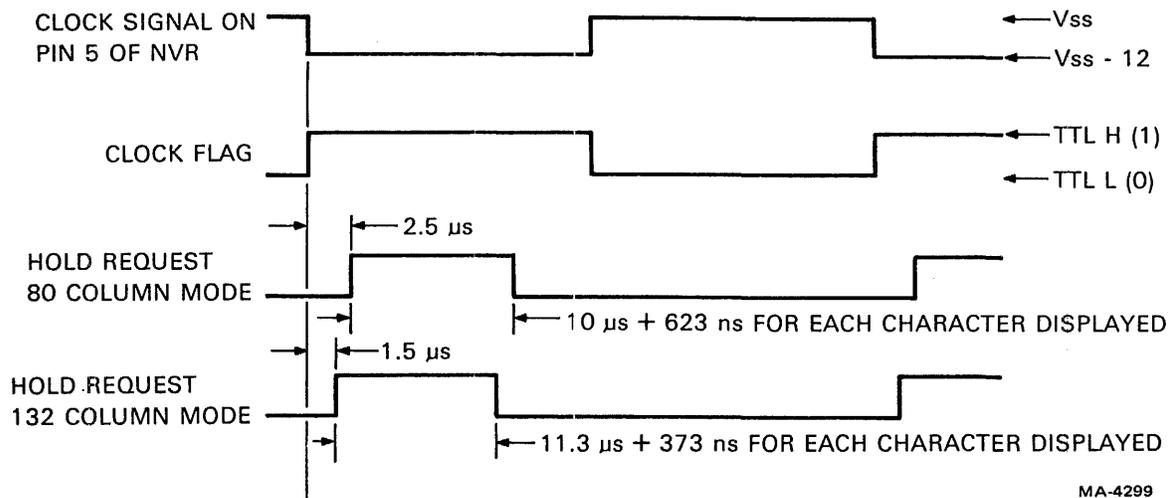
Figure 4-5-2 NVR Signals
