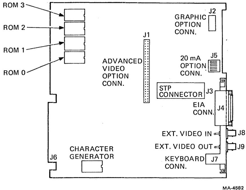
Figure 5-32 Terminal Controller Board
