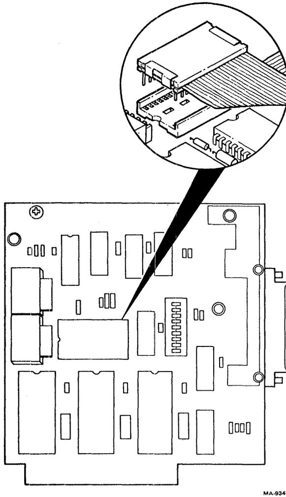
Figure 6-48 24-Pin Flat Cable on STP Board
