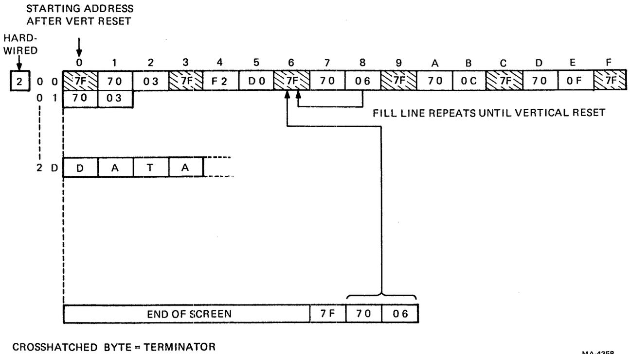
Figure 4-7-7 End of Screen Fill Line Operation
