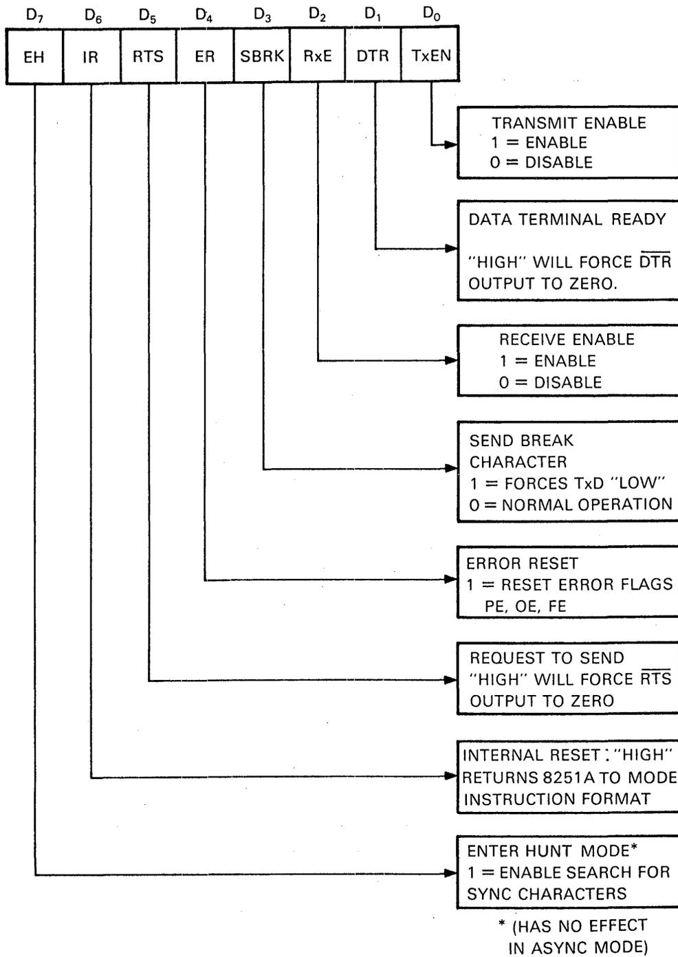
NOTE: ERROR RESET MUST BE PERFORMED WHENEVER RxENABLE AND
