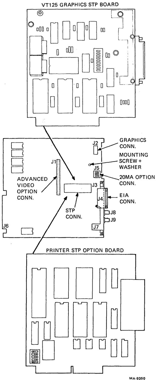
Figure 5-14 Installing Printer Port on VT125 STP Board
