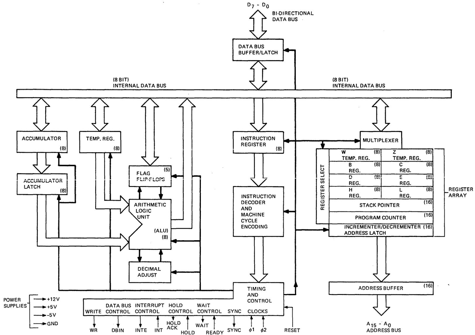
Figure 4-2-1 8080 Block Diagram
