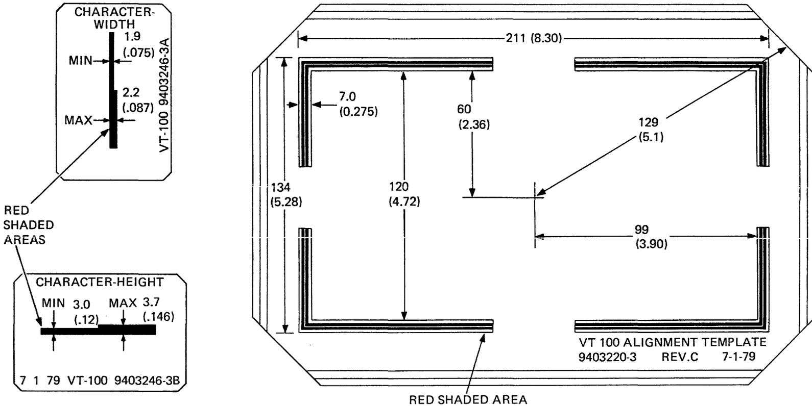
NOTE: MEASUREMENTS ARE IN MILLIMETERS EXCEPT VALUES IN PARENTHESIS ARE IN INCHES.
