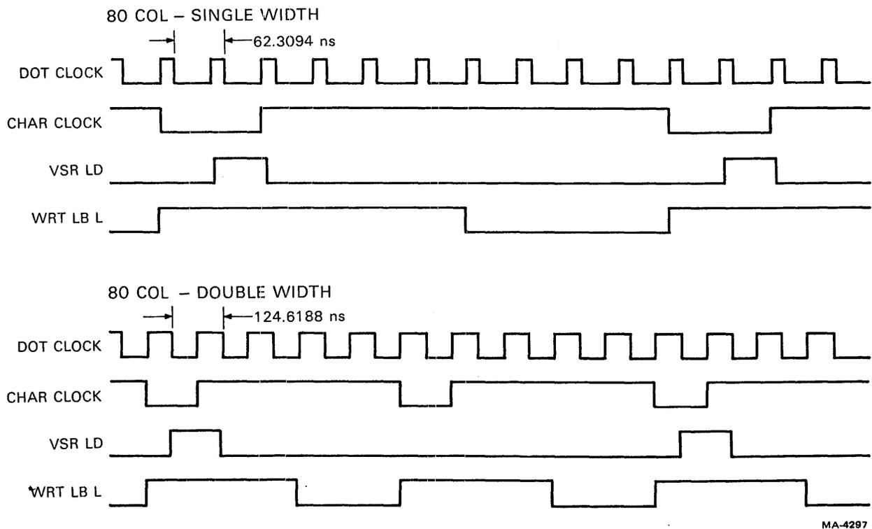
Figure 4-6-6 Video Latch Timing – 80 Column
