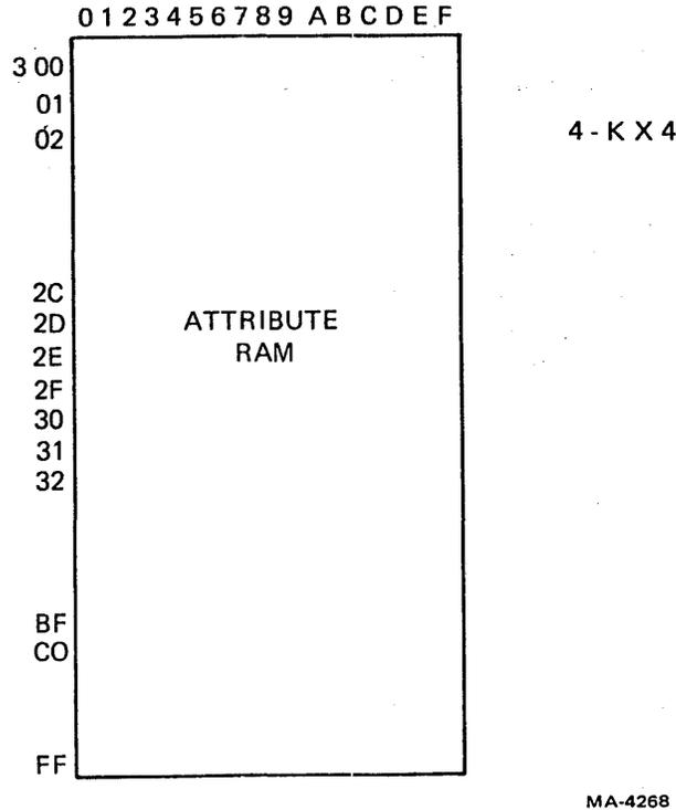
Figure 4-7-3 Screen RAM Organization – 80 Column, 60 Hz
