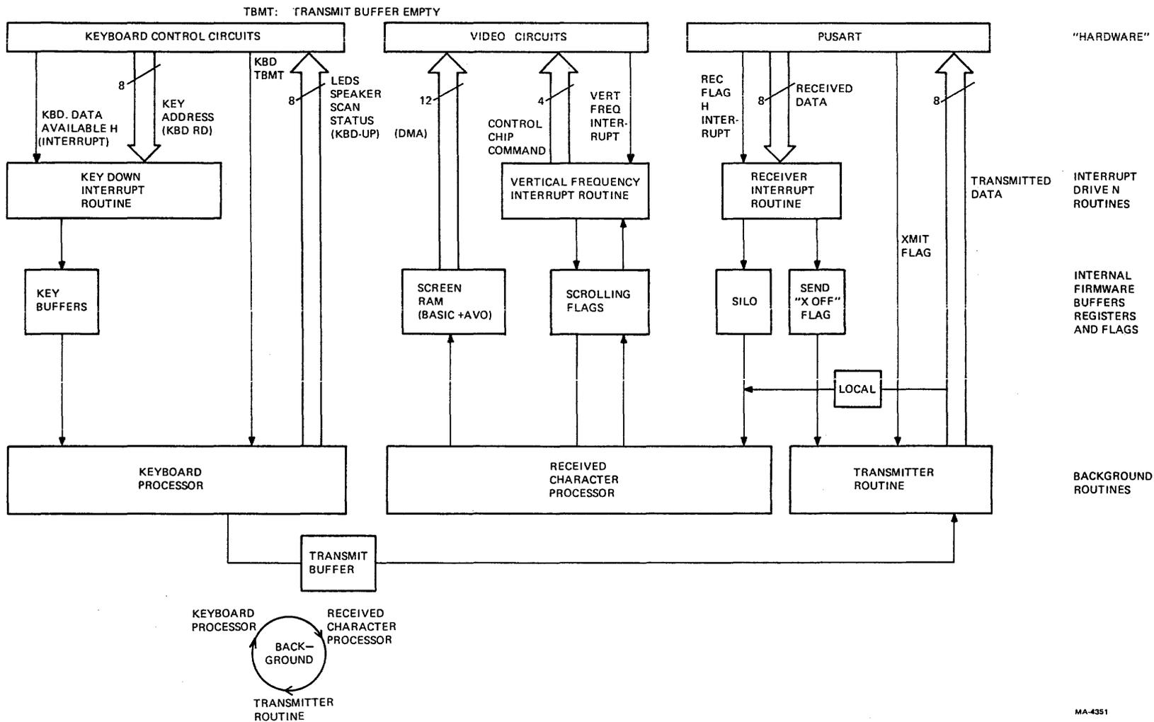
Figure 4-1-3 VT100 Firmware Block Diagram
