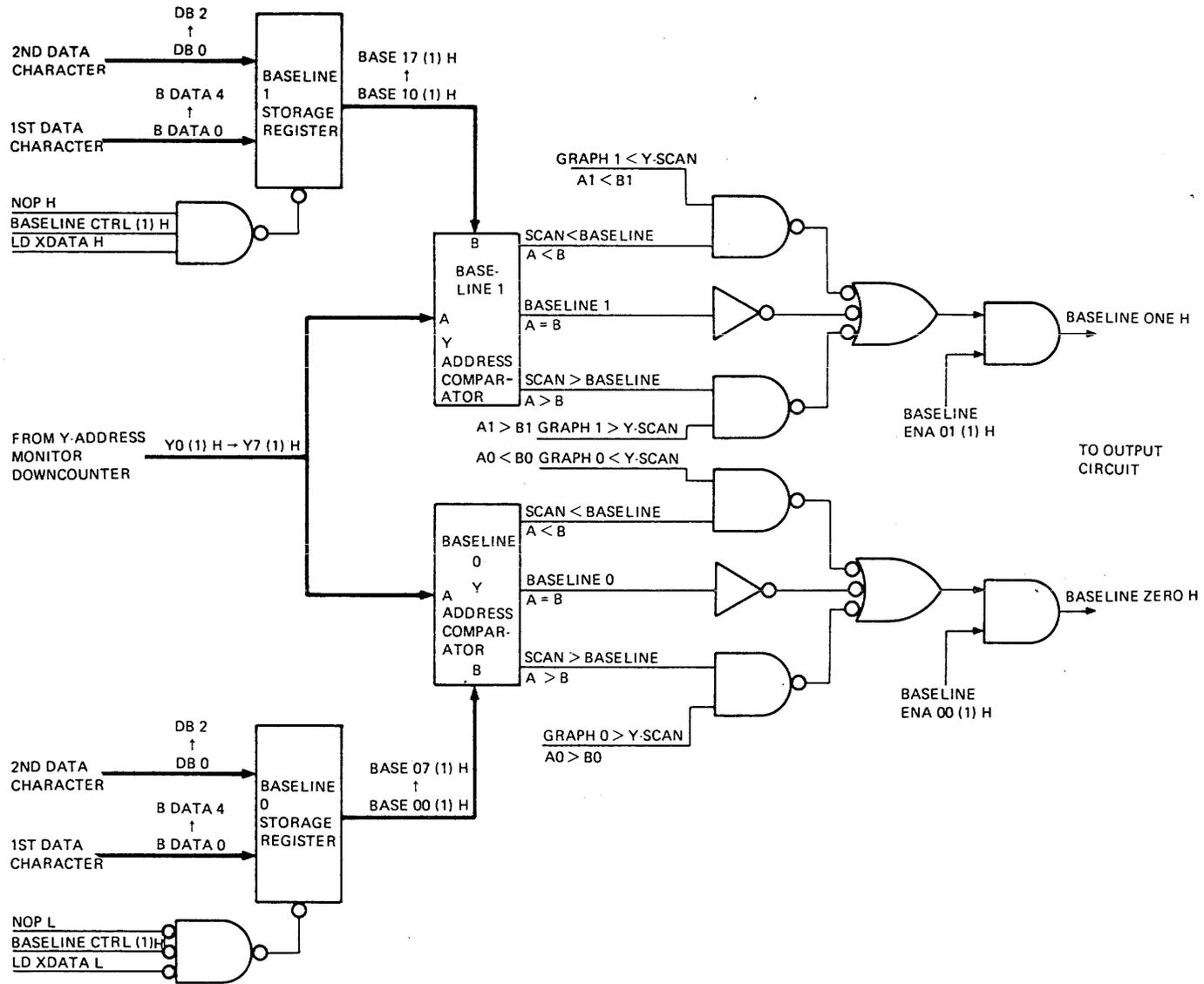
Figure 6-29 Baseline (Shade Line) Registers and Comparators
