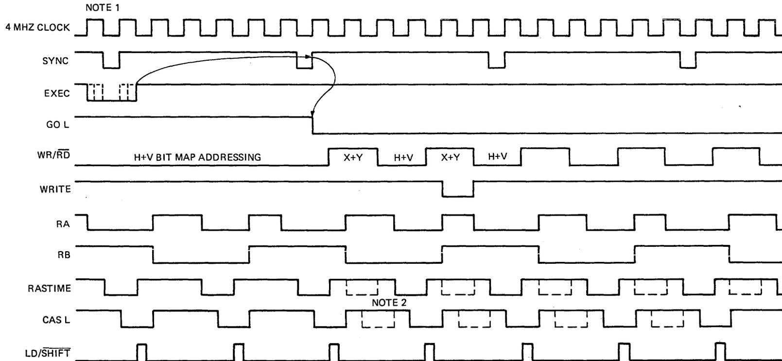
NOTE 1 SIGNALS ARE LATCHED BY 8 MHZ. 1/2 CYCLE SHIFT NOT SHOWN.
