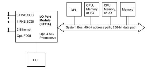
The AlphaServer 8200 has a five-slot system bus. The minimum system configuration is one CPU module (with one or two CPUs), one memory module, and one I/O adapter. The KFTIA I/O port module is shown in this block diagram. The remaining two slots in the backplane can be used for CPU, memory, or I/O adapters, either the KFTIA or the KFTHA.
