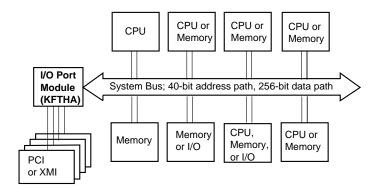
The AlphaServer 8400 has a nine-slot system bus. The minimum system configuration is one CPU module (with one or two CPUs), one memory module, and one I/O adapter. The I/O adapter shown here is the KFTHA. The remaining slots in the backplane can be used for CPU, memory, or KFTHA or KFTIA I/O adapters, within the following limits:
