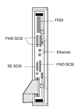
Figure 7 KFTHA Module with Four Channels
