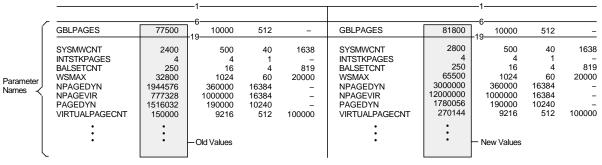
Make any adjustments in MODPARAMS.DAT using symbols prefixed by MIN\_, MAX\_, or ADD\_. For example, if AUTOGEN calculated a smaller value for GBLPAGES, you might specify a minimum value for this parameter as follows:
