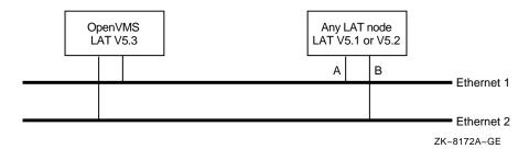
Any configuration similar to this diagram will result in unpredictable results and may not function. In a network environment, LAT Version 5.1 and 5.2 nodes can have only a single logical LAN address. The configuration in Figure 26–5 violates this rule. The configuration shown in Figure 26–4 is a valid alternative.
