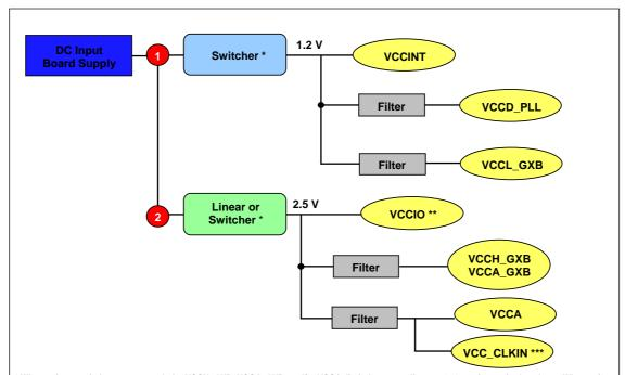
\* When using a switcher power supply for VCCH\_GXB, VCCA\_GXB, and/or VCCA, limit these supplies to ± 3 % maximum ripple voltage. When using a switcher power supply for VCCD\_PLL, and/or VCCL\_GXB, limit these supplies to ± 3 % maximum ripple voltage.
